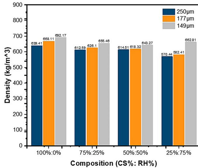
Figure 2. Density versus composition with different particle sizes
