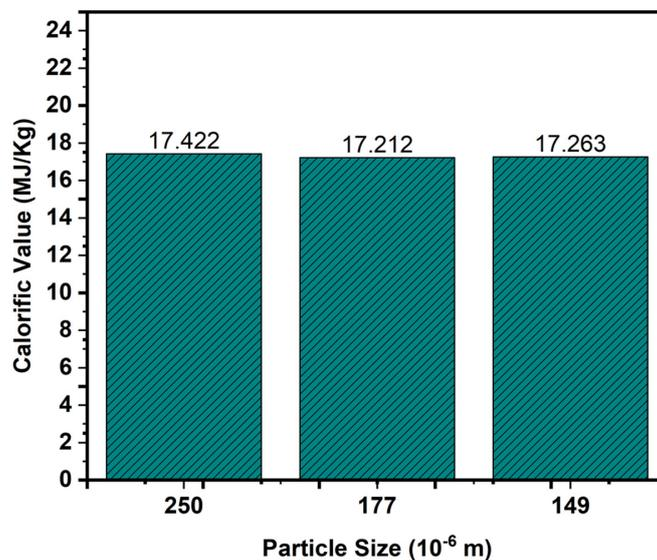
Figure 9. Calorific value against different particle sizes with the composition of 25%:75% (CS: RH)
