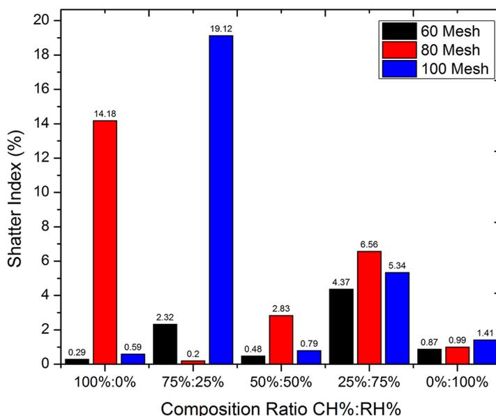
Figure 7. Shatter index versus composition under different particle sizes
