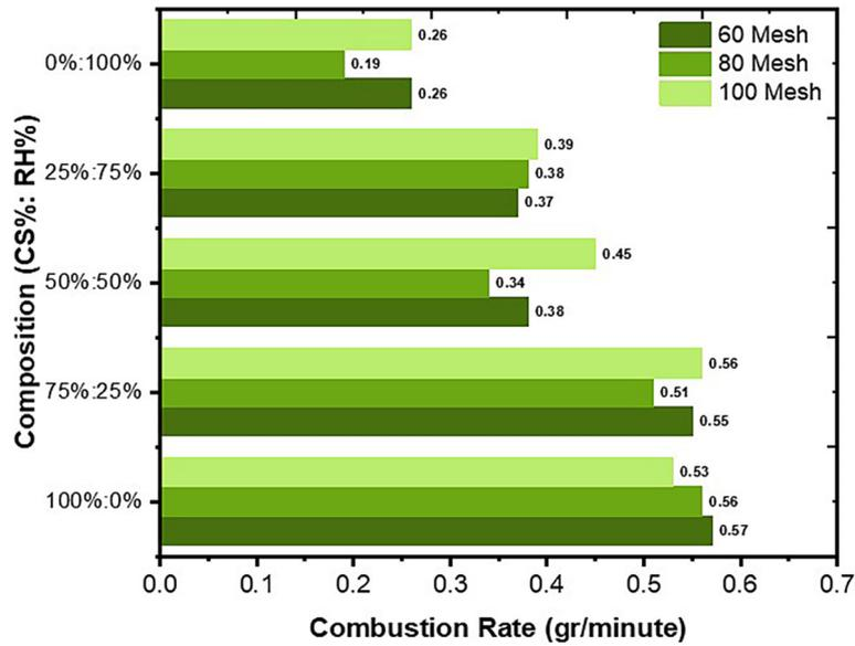
Figure 8. Combustion rate versus composition under different particle sizes
