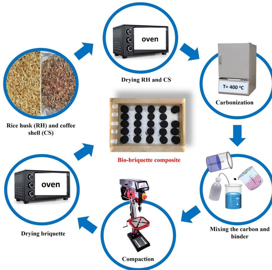
Figure 1. Briquetting procedure
