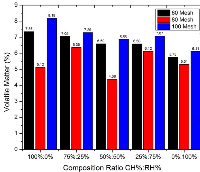
Figure 4. Volatile matter versus composition under different particle sizes
