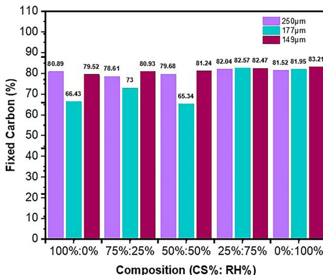
Figure 6. Fixed carbon versus composition under different particle sizes
