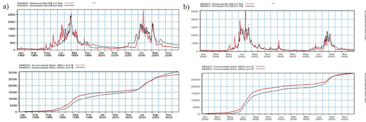
**Fig. 2.** Discharge and yearly accumulated water volume in Nam Ou River at the station Muong Ngoy for the (a) calibration period, and (b) validation period
