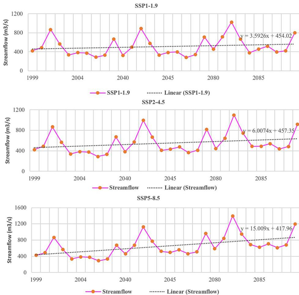
Fig. 4. The annual streamflow simulated by the calibrated MIKE-NAM model for 2020–2099 under the SSP1-1.9, SSP2-4.5, and SSP5-8.5 scenarios
