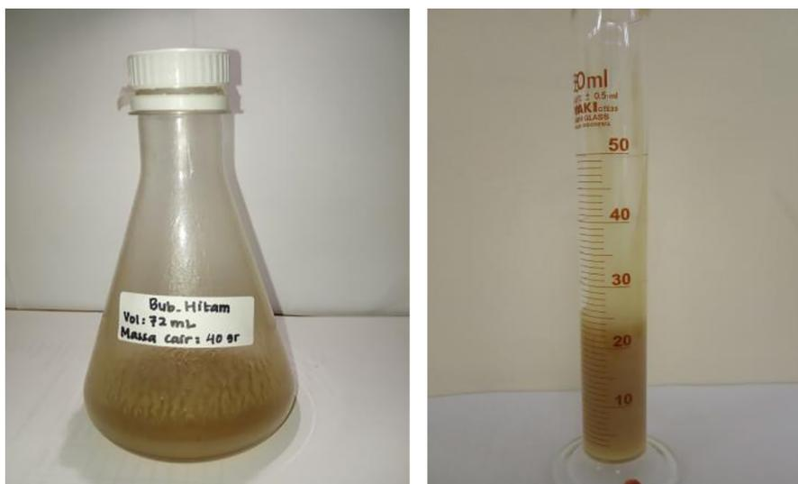
**Figure 3.** Pyrolysis oil products from plastic bubble wrap (a) and plastic packaging (b)
