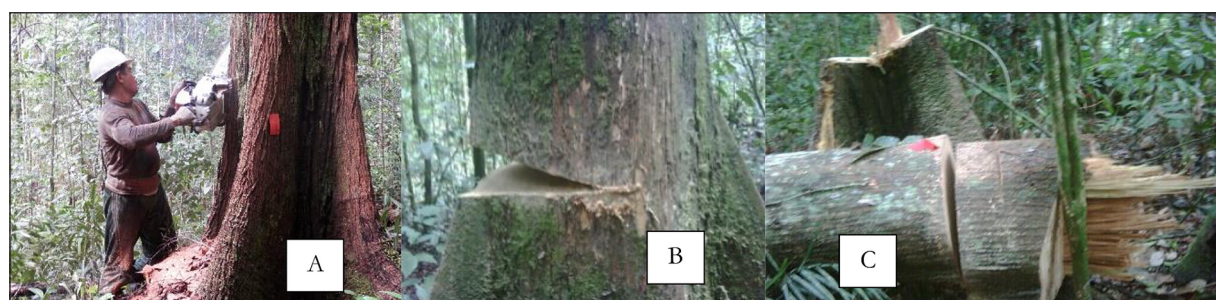
Figure 2. Technical errors in logging trees in natural forest: A = cutting too high, B = small notch size (< 450), C= uprooted fiber at the base of the stem
