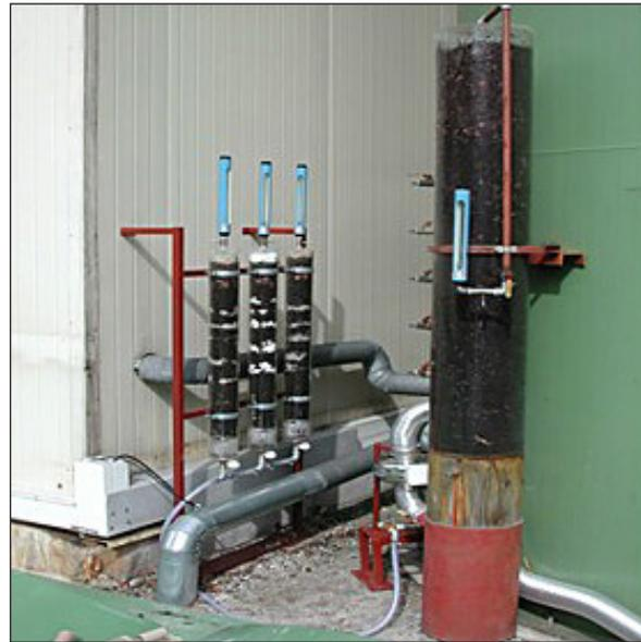
**Figure 1.** Test rig for deodorisation of industrial gases using peat-bark filled biofilters and biofilters with plant fibre layers
