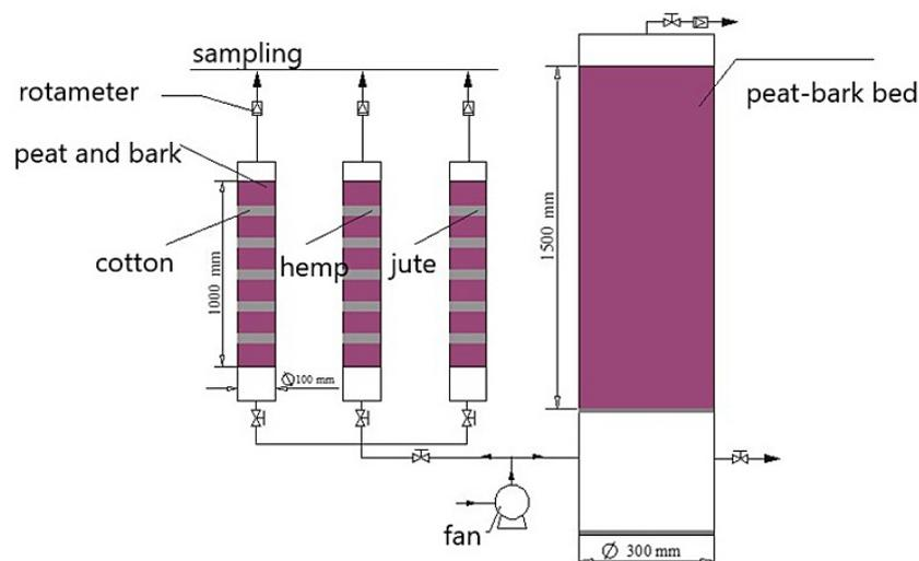
**Figure 2.** Schematic diagram of the test rig consisting of biological beds filled with a mixture of peat and bark, jute, hemp and cotton
