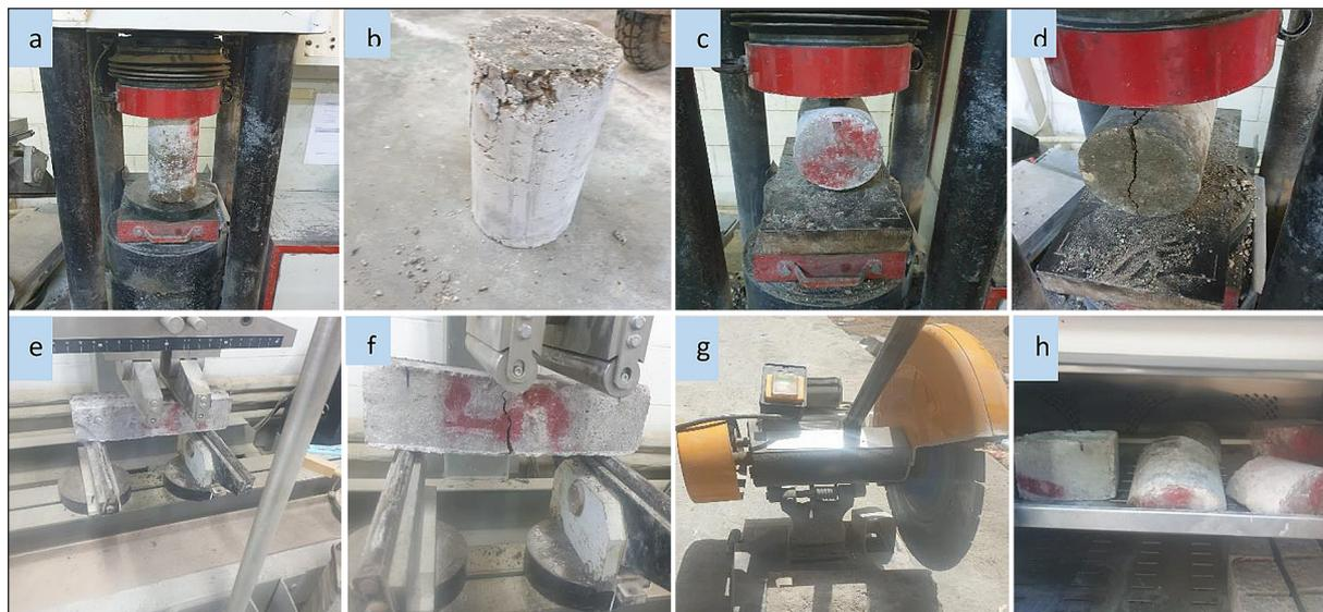
**Figure 4.** (a) Specimen in compressive-test machine (b) Specimen after failure due to compressive stress (c) Specimen in splitting test machine (d) Specimen after failed due to tensile stress (e) Specimen in flexural testing machine (f) Specimen after failure due to flexural stress (g) Cutting the specimens, and (h) Drying the specimens for 1 day
