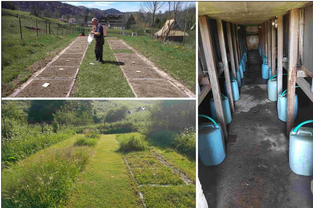
**Figure 2.** Above-ground and underground part of the experimental structure with the lysimeters (photo by Jaguś & Kowalczyk)
