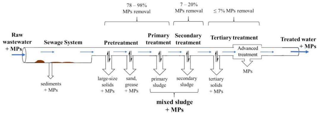
Figure 6. WWTP process schematic and MPs removal (Masia et al., 2020)
