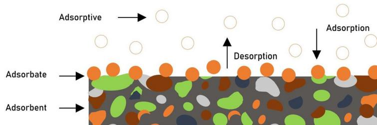
Figure 1. Adsorption mechanism
