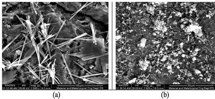
**Figure 9.** Morphology of green sand (2500×): (a) before adsorption, (b) after adsorption
