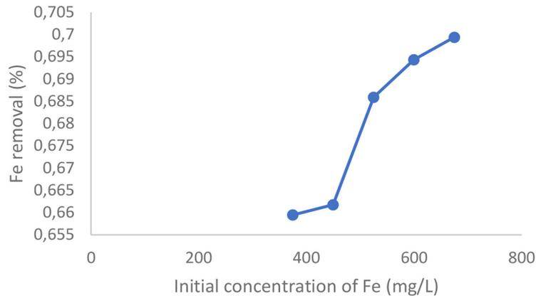
**Figure 2.** The effect of the initial concentration of Fe on the percentage of Fe adsorption
