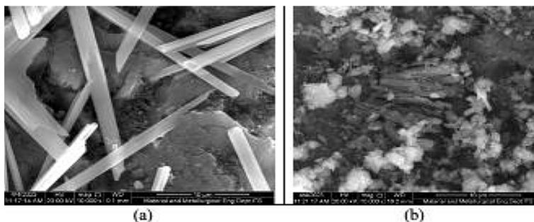
**Figure 11.** Morphology of green sand (10000×): (a) before adsorption, (b) after adsorption
