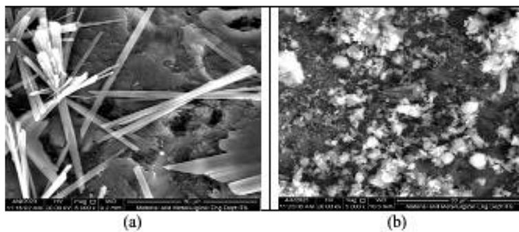
**Figure 10.** Morphology of green sand (5000×): (a) before adsorption, (b) after adsorption
