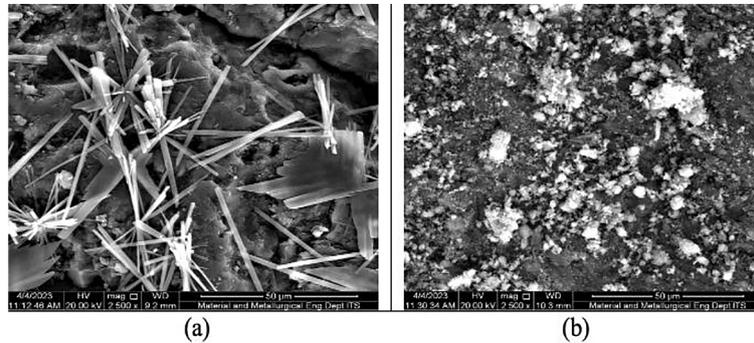
**Figure 8.** Morphology of green sand (1000×): (a) before adsorption, (b) after adsorption
