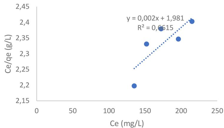
**Figure 7.** Langmuir adsorption isotherm model for Mn
