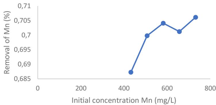
**Figure 3.** The effect of the initial concentration of Mn on the percentage of Mn adsorption
