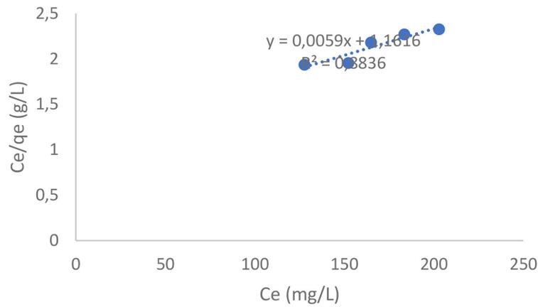
**Figure 5.** Langmuir adsorption isotherm model for Fe
