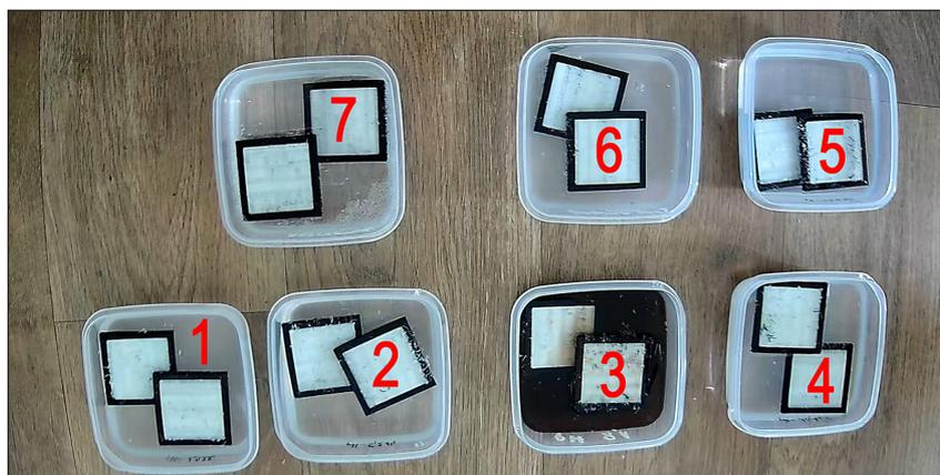
**Fig. 6.** The process of dissolving BVOH in aqueous solutions
