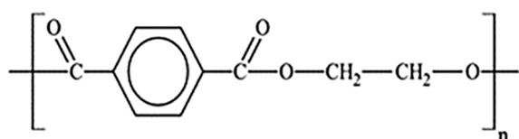
Fig. 1. Chemical structure of PETG copolymer
