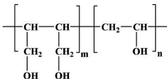
Fig. 2. Chemical structure of BVOH molecules
