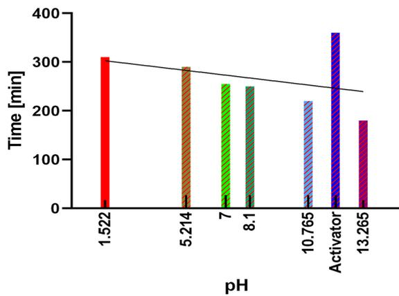
Fig. 8. Average dissolution time of BVOH in the tested samples
