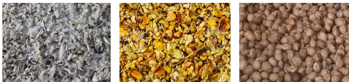
Figure 1. Agri-food industry plant waste groups selected for study: (a) sugar beet marc, SBSF; mixed vegetable waste, MVW; (c) cherry stones, ChS
