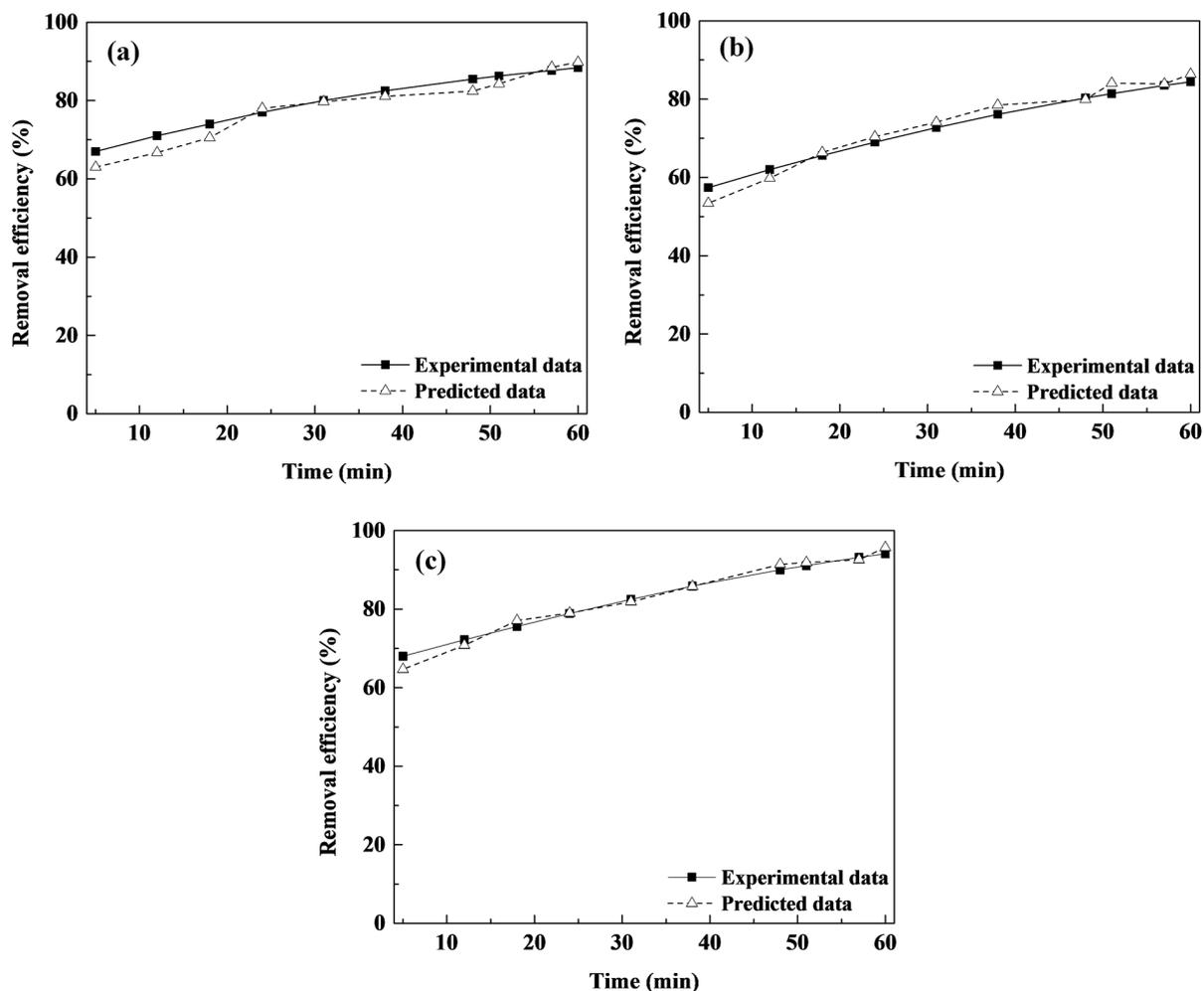
**Figure 4.** Experimental results and predicted output from GCNN at different speeds UV intensities (a) 0, (b) 20, and (c) 40 W
