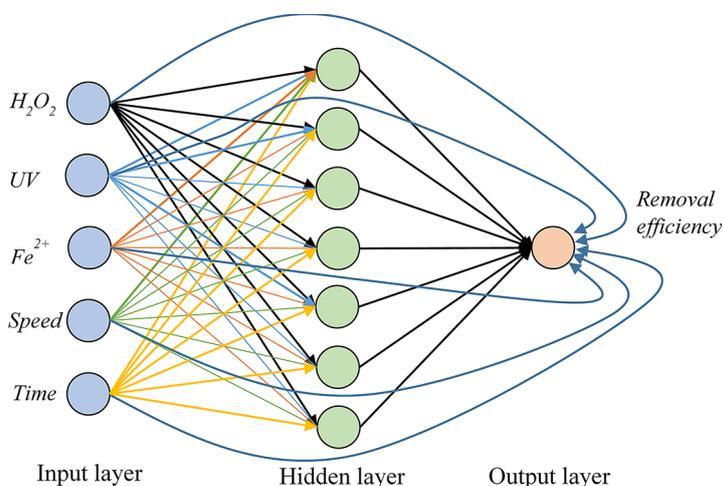
**Figure 1.** Suggested cascade-forward neural network for predicting the output of removal efficiency from the inputs of  $H_2O_2$ , UV,  $Fe^{2+}$ , mixing speed, and contact time
