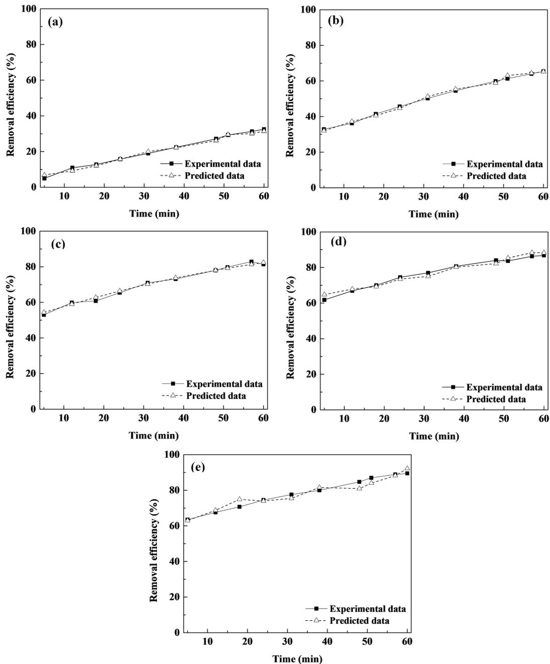
**Figure 5.** Experimental results and predicted output from GCNN at different  $\text{Fe}^{2+}$  concentrations (a) 0, (b) 0.4, (c) 1, (d) 1.65, and (e) 2.33 mM/L
