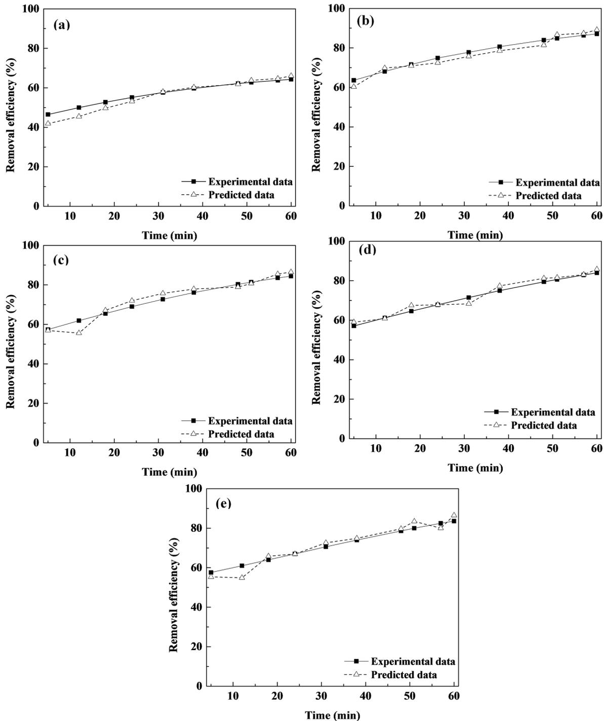
**Figure 3.** Experimental results and predicted output from GCNN at different  $H_2O_2$  concentrations (a) 0, (b) 0.5, (c) 1.5, (d) 3, and (e) 5 mM/L
