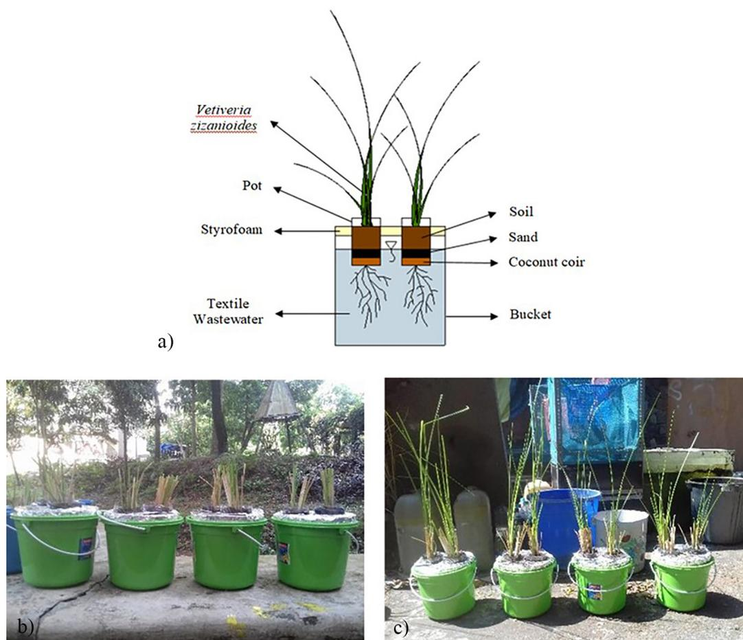
**Fig. 1.** Experimental setup of floating treatment wetland reactor (a), beginning of acclimatization (b), after 30 days acclimatization (c)
