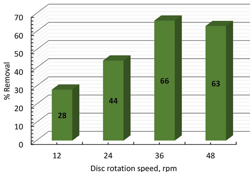
Fig. 5. Effect of disc rotation speed on the removal efficiency of dodecane
