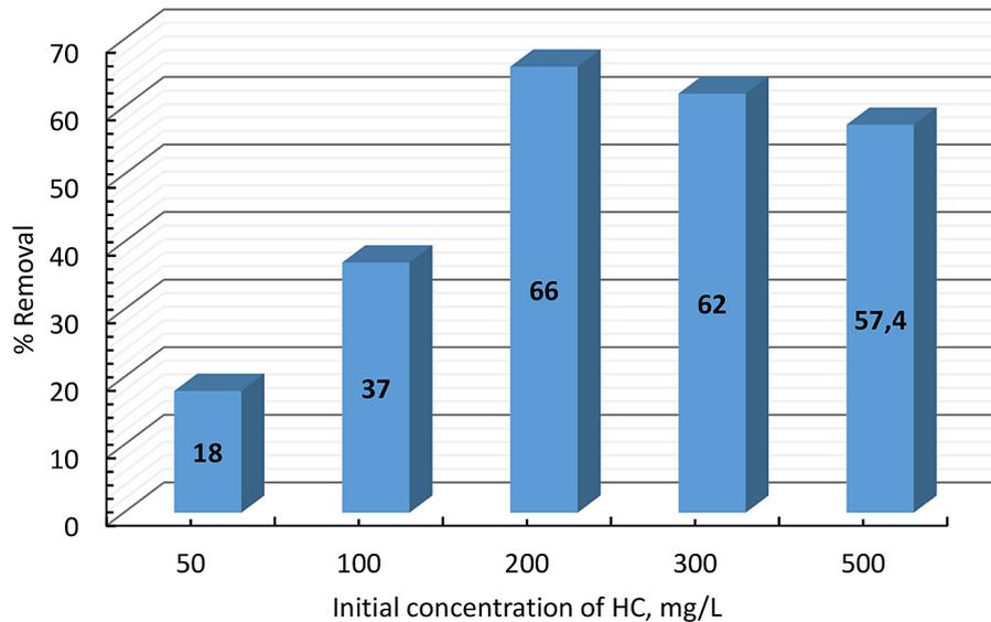
**Fig. 2.** Effect of initial concentration of HC on removal efficiency (disc rotation speed = 48 rpm; biomass dosage = 1000 mg/L; contact time = 84 min.)
