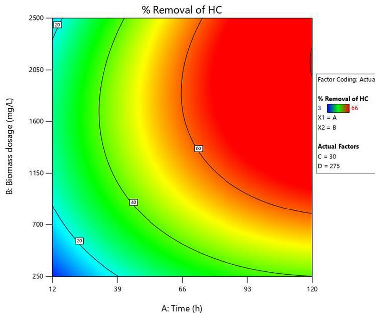
Fig. 7. Contour plot of % removal of HC dodecane at different contact times and biomass dosages
