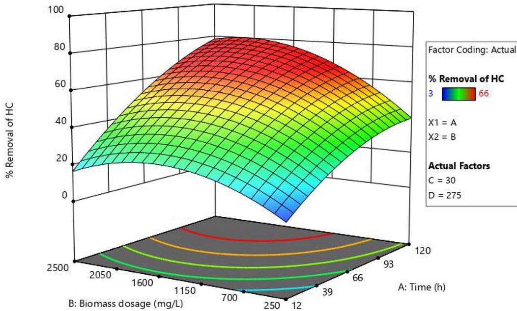
Fig. 6. 3D response plot of % removal of HC dodecane at different contact times and biomass dosages
