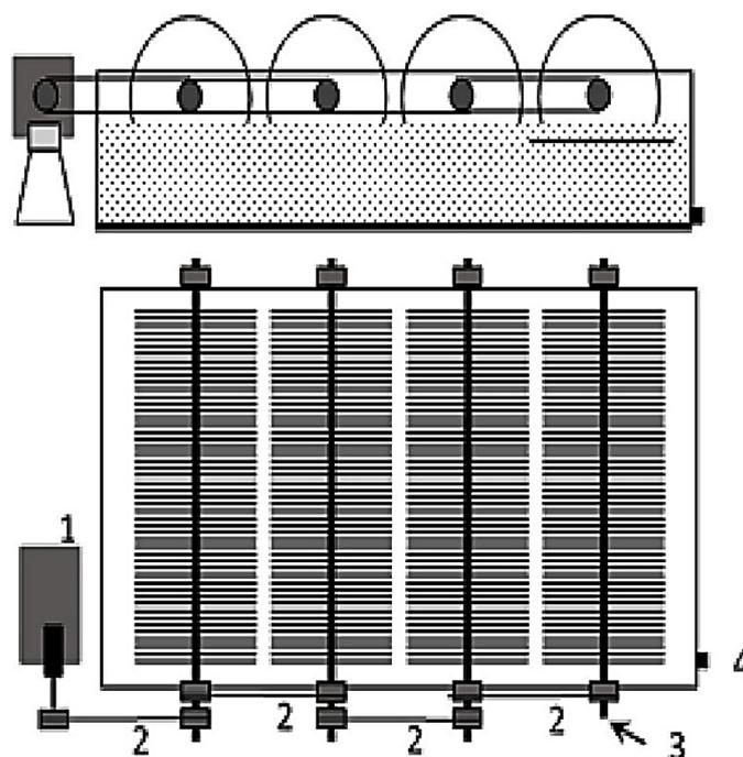
Fig. 1. Schematic diagram of RBC reactor: (1) drive motor; (2) belt conveyer; (3) shaft; (4) drain
