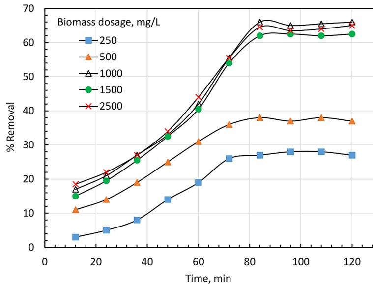
Fig. 3. Removal efficiency vs. time at different biomass dosages (initial concentration of HC = 200 mg/L, disc rotation speed = 48 rpm)
