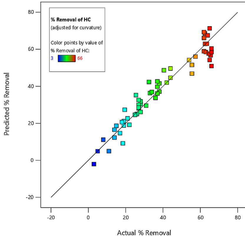
**Fig. 8.** Comparison of the experimental results and the obtained reduced quadratic model Equation 1
