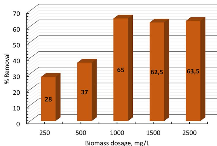
Fig. 4. Removal efficiency vs. biomass dosage (initial concentration of HC = 200 mg/L; disc rotation speed = 48 rpm; contact time = 96 min.)
