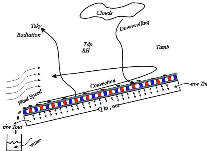
Figure 6. Schematic of VAR natural radiative cooling AWH technique
