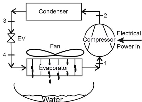
**Figure 3.** Schematic of VCR AWH technique
