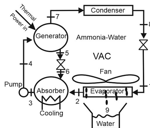
Figure 4. Schematic of VAR AWH technique
