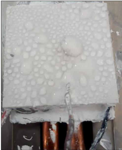
**Figure 2.** Thermoelectric water harvester with enhanced heat transfer rate
