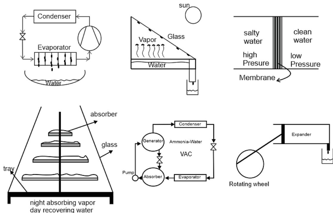
Figure 1. Schematic diagrams of various water harvesting systems
