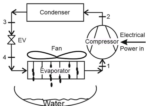
**Figure 3.** Schematic of VCR AWH technique
