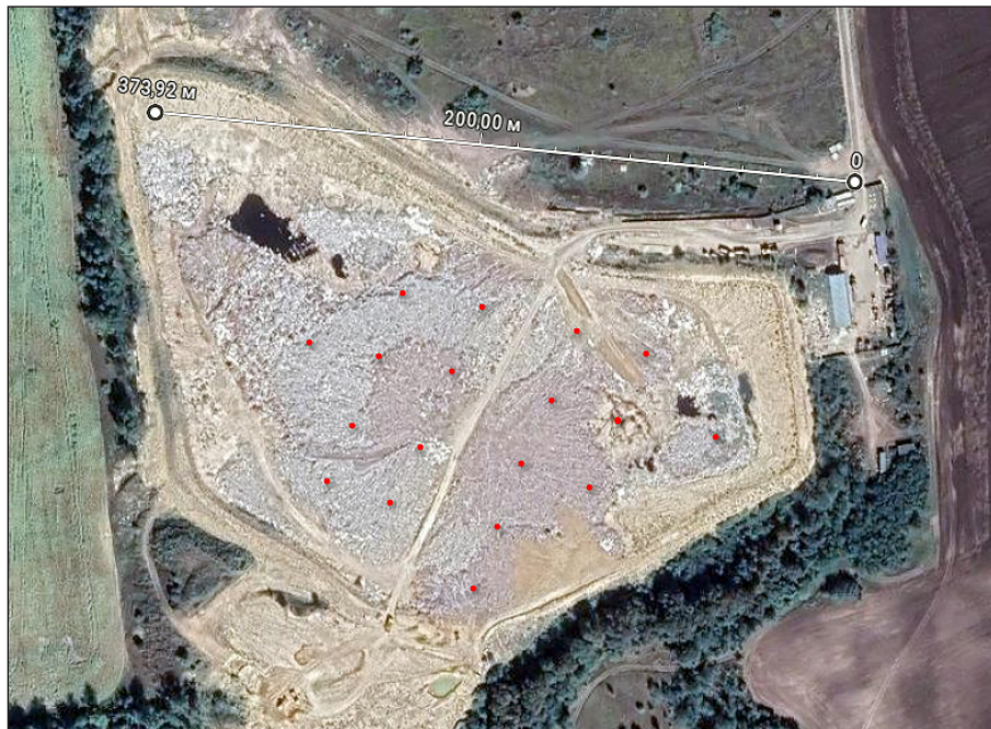
Figure 6. Scheme of degassing wells on the Sumy City landfill (placed based on the satellite image)
