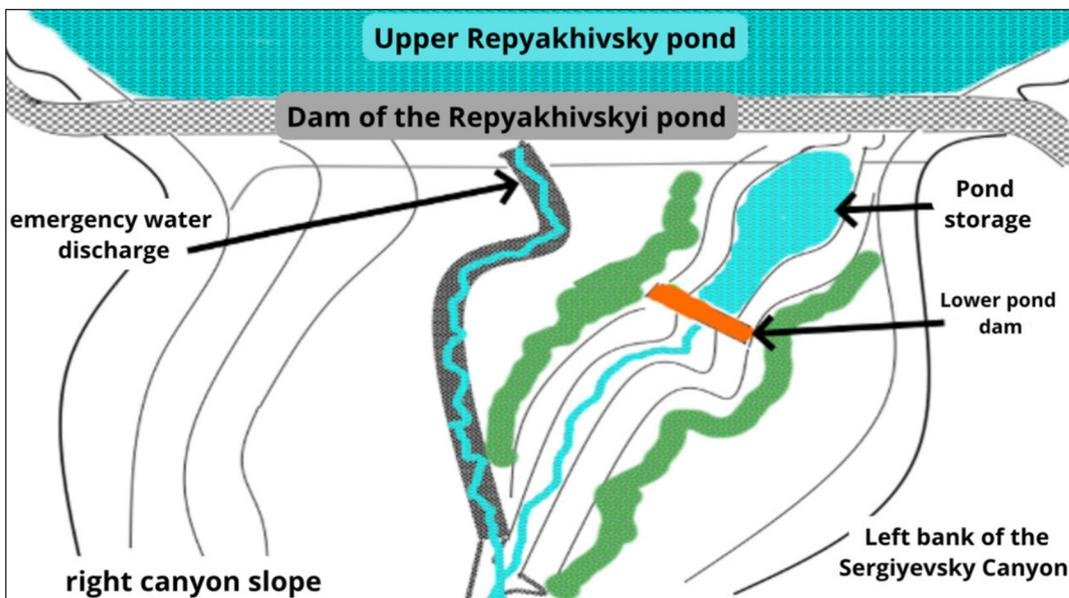
**Fig. 6.** The upper and lower ponds and their spillways within Serhiyivka Canyon
