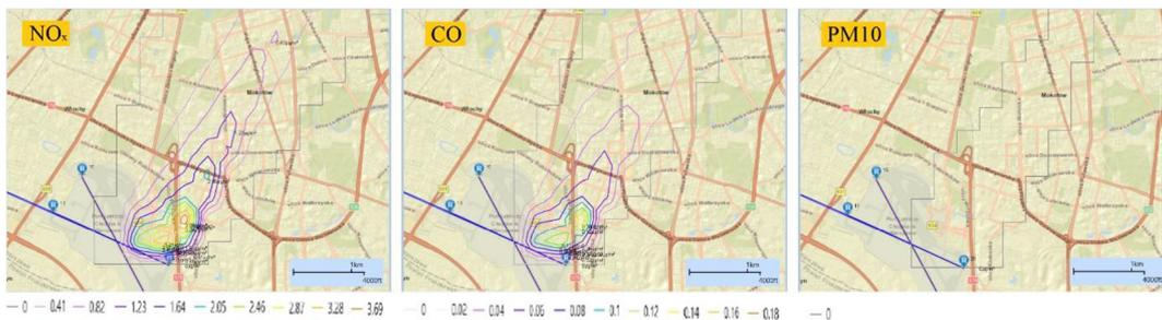
**Figure 11.** The results of pollutant dispersion simulation on January 18 (results given in  $\mu\text{g}/\text{m}^3$ )
