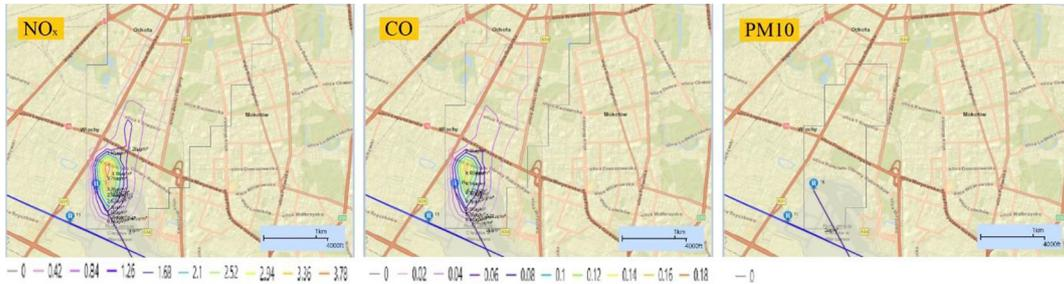
**Figure 9.** The results of pollutant dispersion simulation on January 10 (results given in  $\mu\text{g}/\text{m}^3$ )
