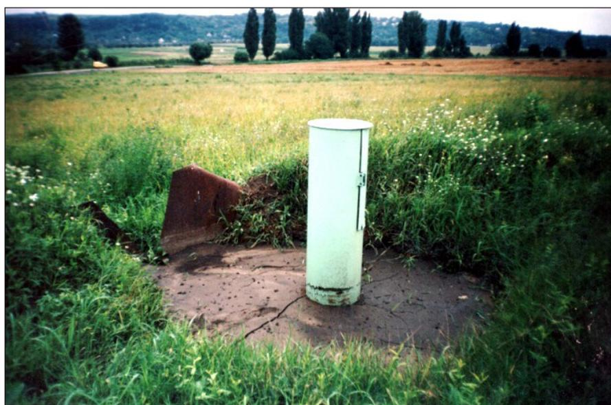
**Figure 4.** Automatic run-off recorder in run-off site of field experiment
