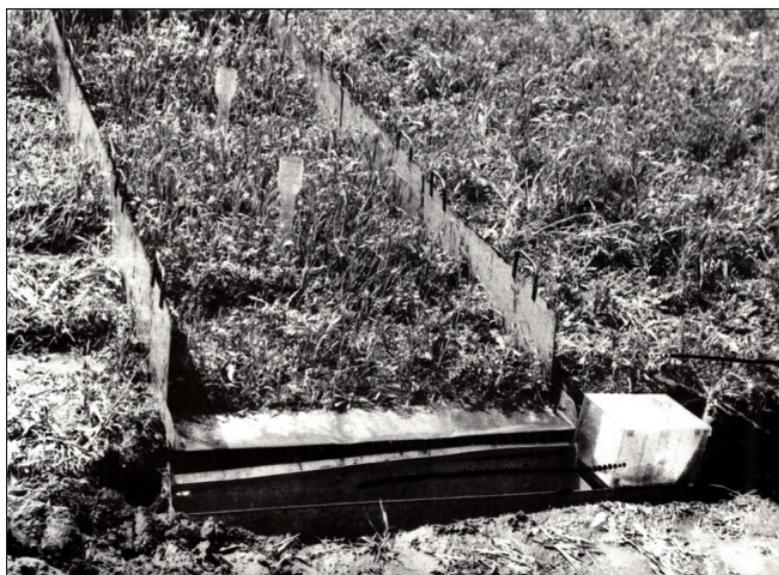
**Figure 8.** Model run-off plot with artificial sprinkling equipped with automatic run-off recording unit in exit range
