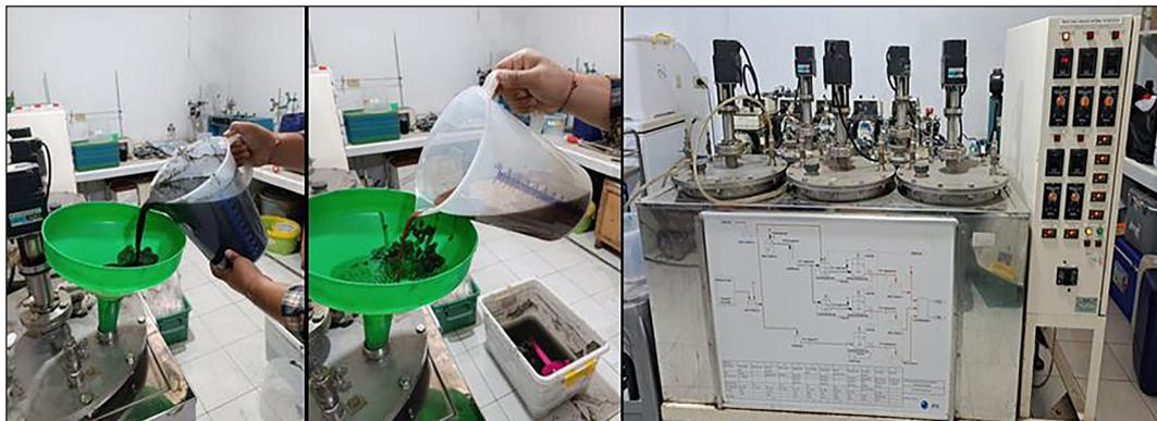
Figure 10. Sludge (a) and POME (b) added in Stirrer tank anaerobic reactor (c)
