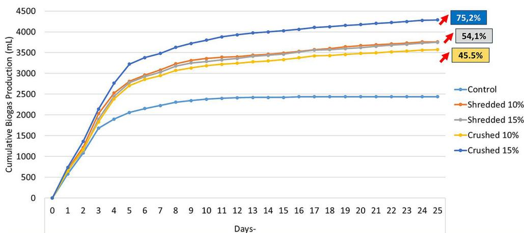
Figure 15. Cumulative biogas production
