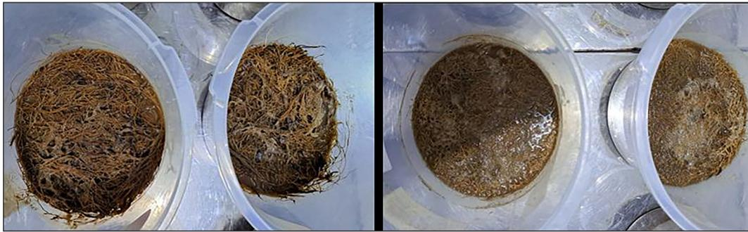
Figure 4. Soaking shredded (a) and crushed (b) EFB in POME
