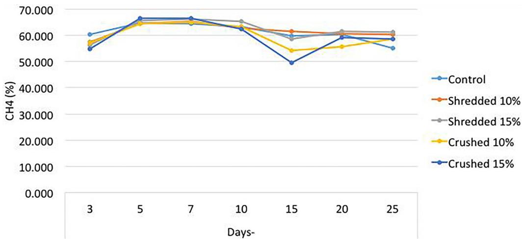
Figure 16. Methane content in the biogas from anaerobic reactor
