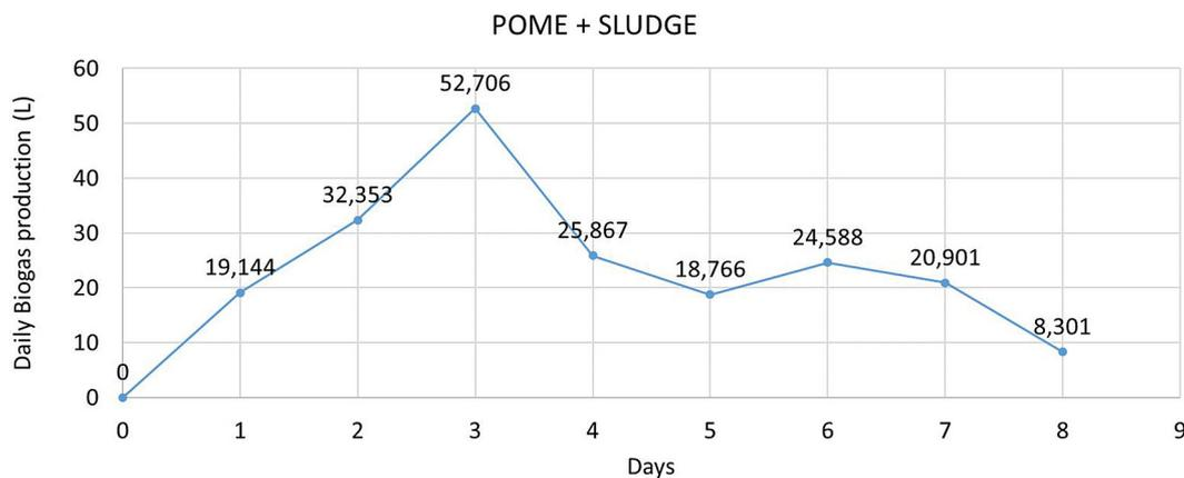
Figure 11. Daily biogas production during acclimatization
