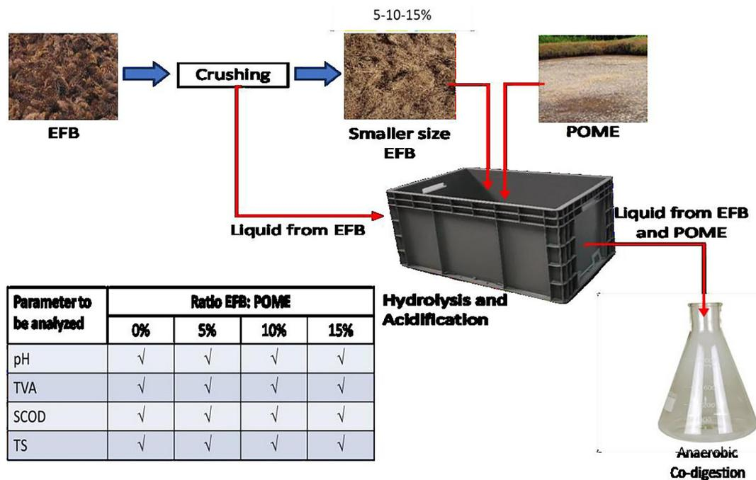
Figure 1. Pre-treatment of EFB and POME before anaerobic co-digestion
