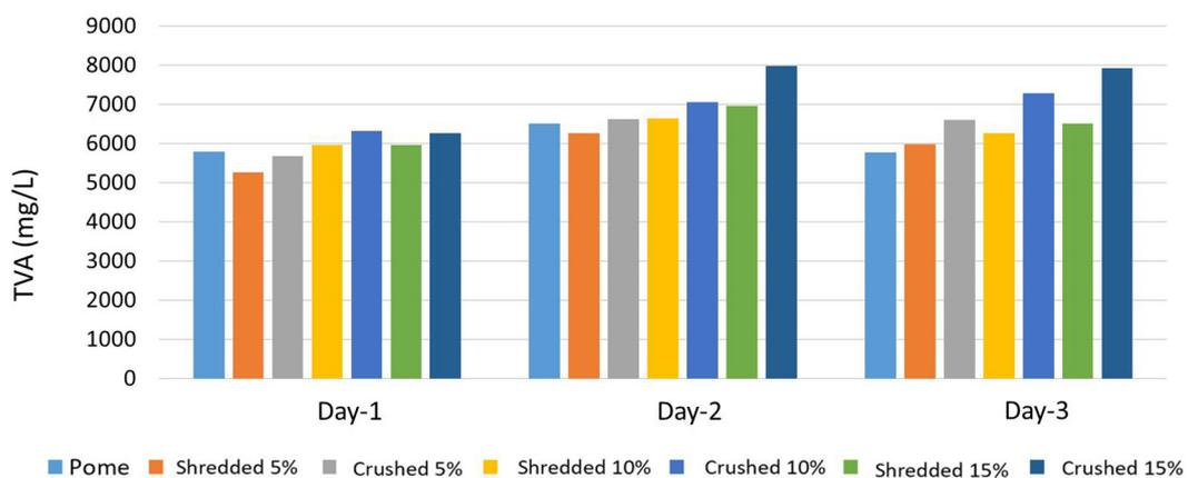
Figure 8. Total volatile acid analysis on EFB-POME co-digestion pre-treatment
