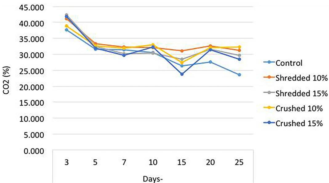
Figure 17. Carbon dioxide content in the biogas from anaerobic reactor
