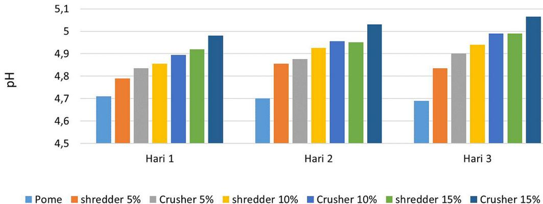
Figure 6. The results of pH analysis on EFB-POME co-digestion pre-treatment
