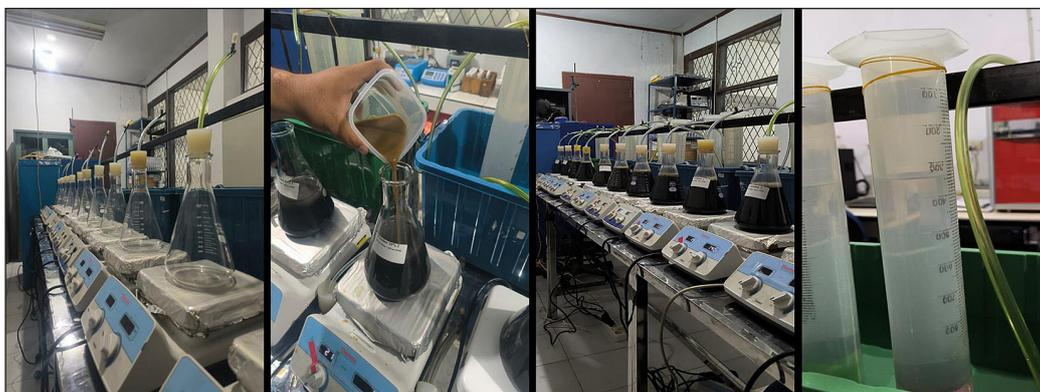
**Figure 13.** Co-digestion of EFB and POME; (a) Erlenmeyer flash reactor before added sludge, (b) Mixing sludge and POME after pre-treatment, (c) Erlenmeyer flash anaerobic reactor, (d) conventional biogas measurement
