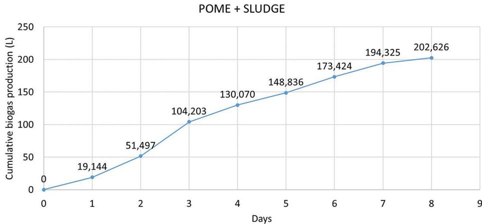
**Figure 12.** Cumulative biogas production during acclimatization
