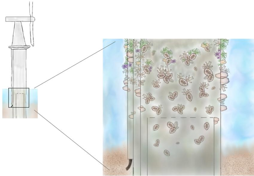
**Figure 1.** A depiction of a biofouling gradient on a monopile. Diversity of the biofouling community decreases with depth. Algae dominants at the air/water interface, hard fouling is abundance at midpoint regions, with biofilm and sometimes hydroids typifying the community close to the seafloor
