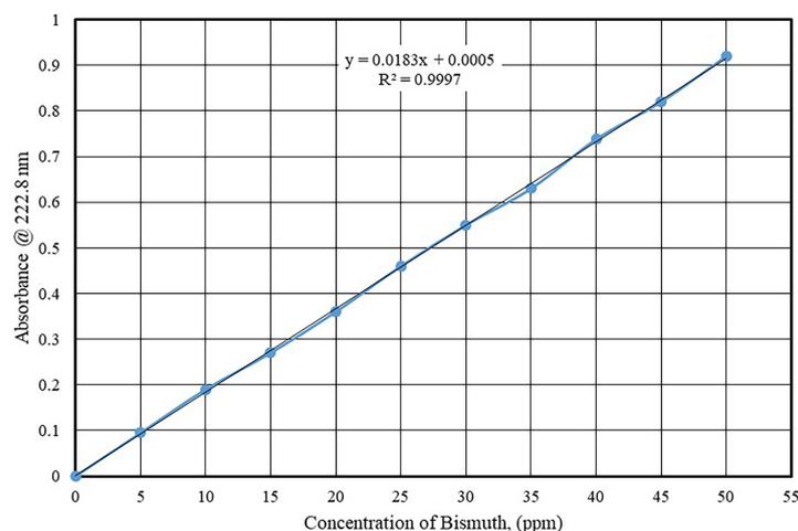
Figure 1. Calibration curve of bismuth using AAS device at  $\lambda_{\text{max}} = 222.8 \text{ nm}$
