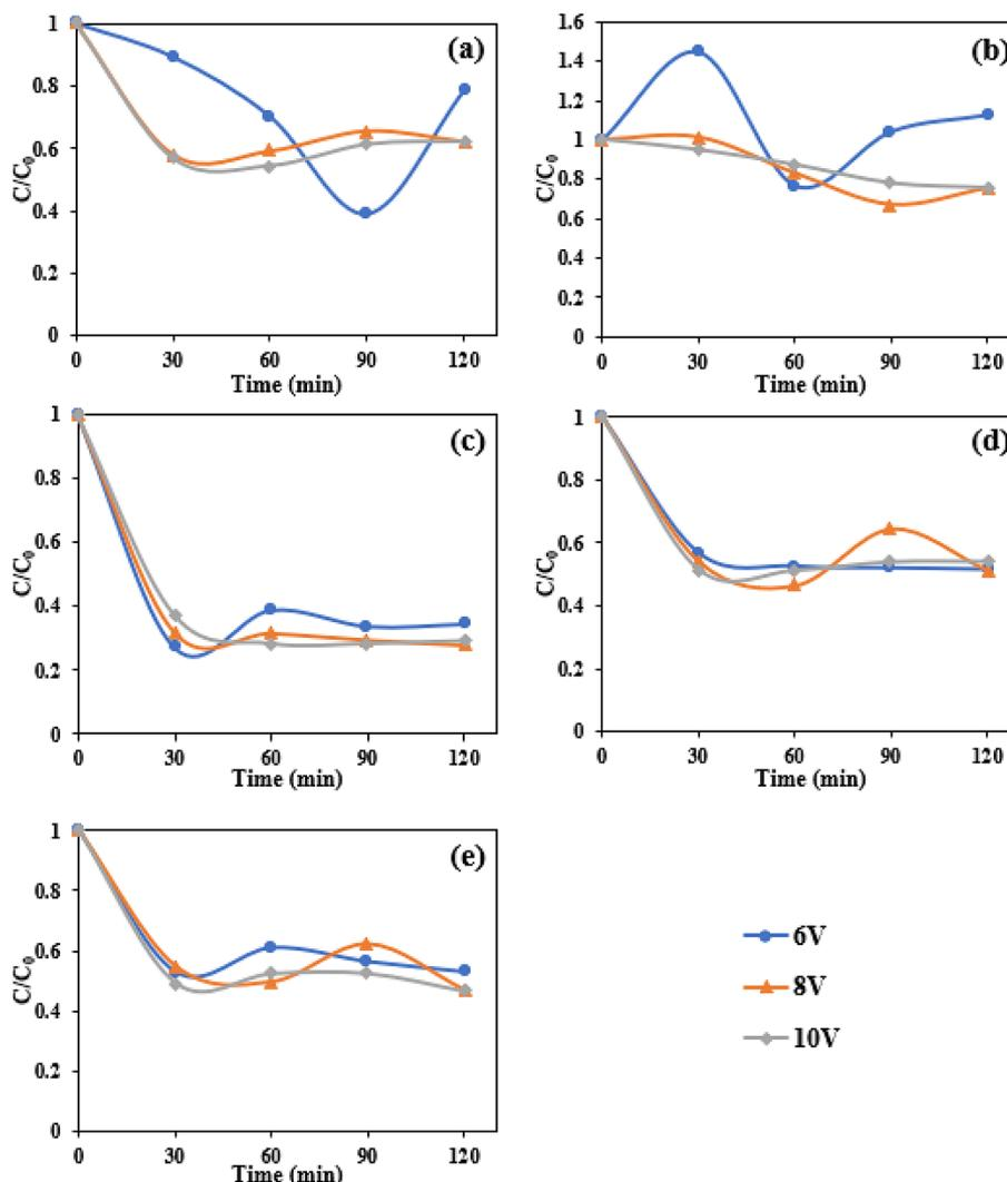
Figure 2. Removal of (a)  $NH_3$ , (b) Cr(III), (c) TSS, (d), BOD, and (e) COD during the electro-Fenton process of leather tannery wastewater
