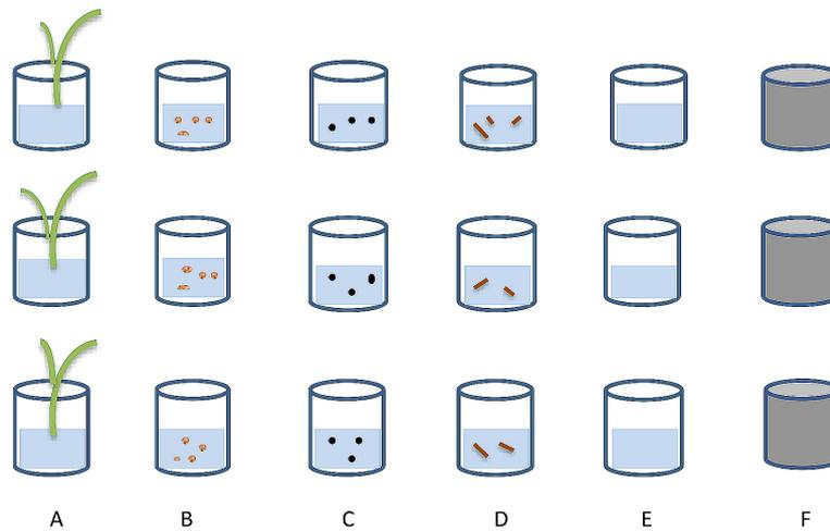
**Figure 1.** Sketch diagram of the hydroponic experiments: (a) hydroponic planted reactors, (b) sand reactors, (c) chicken manure - wood shavings reactors, (d) rhizobacterial-inoculated unplanted reactors, (e) unplanted control reactors, and (f) unplanted dark control reactors
