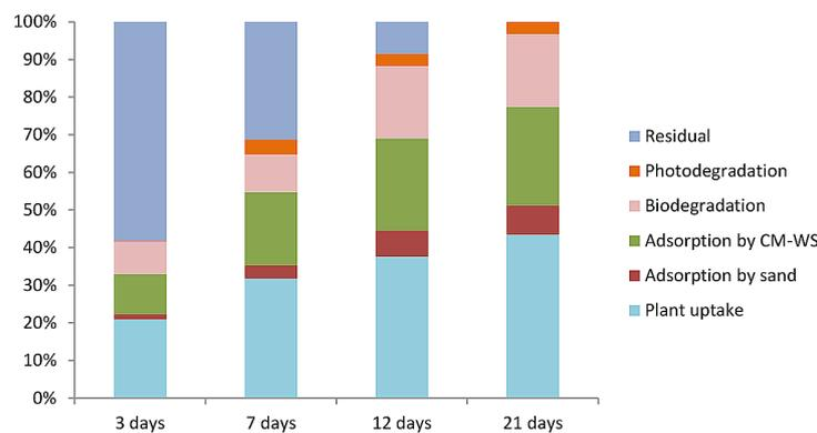
Figure 7. The removal percent of AMX classified as plant uptake, adsorption, biodegradation, photodegradation and residual in the aqueous solution at 4 intervals
