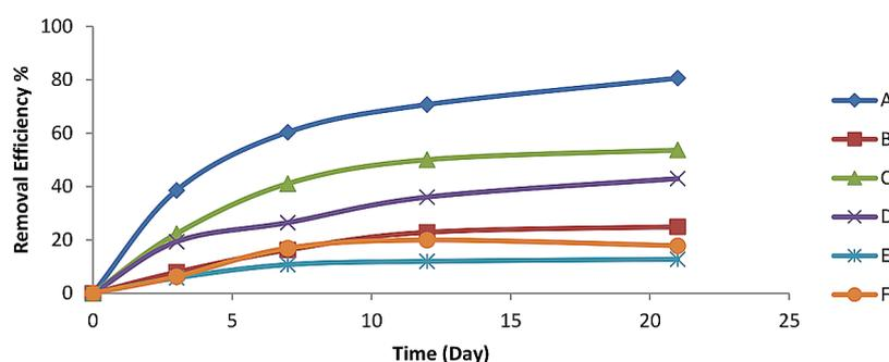
**Figure 4.** Removal of AMX from aqueous solution in the reactors, (a) hydroponic planted reactors, (b) sand reactors, (c) chicken manure - wood shavings reactors, (d) rhizobacterial-inoculated unplanted reactors, (e) unplanted control reactors and (f) unplanted dark control reactors.
