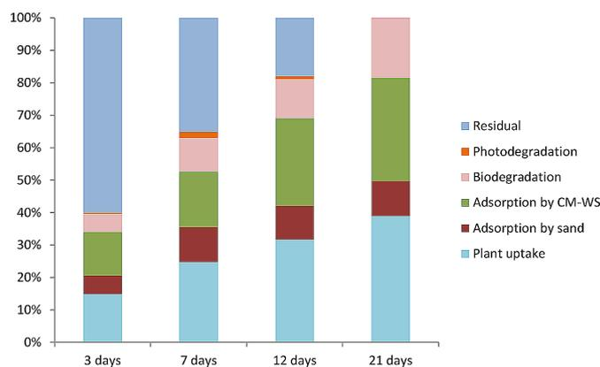
**Figure 8.** The removal percent of CIP as classified plant uptake, adsorption, biodegradation, photodegradation and residual in the aqueous solution at 4 intervals
