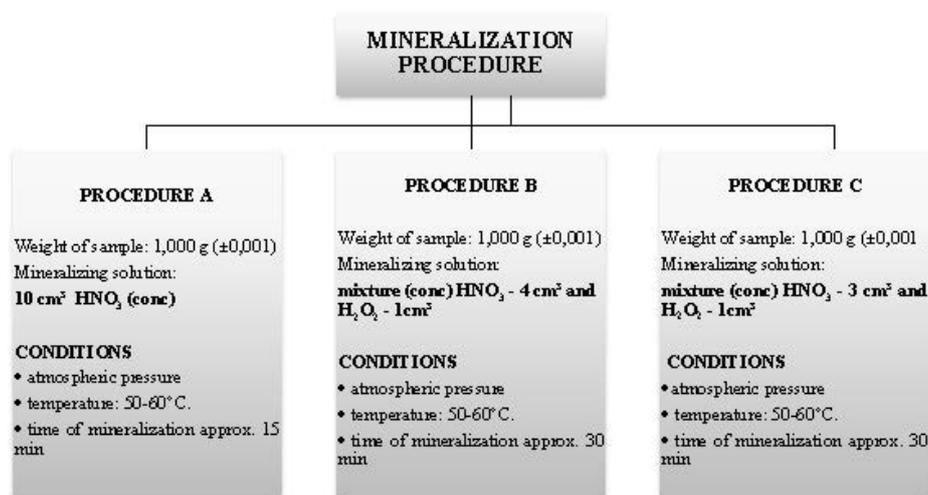
Figure 1. The detailed conditions of mineralization procedures
