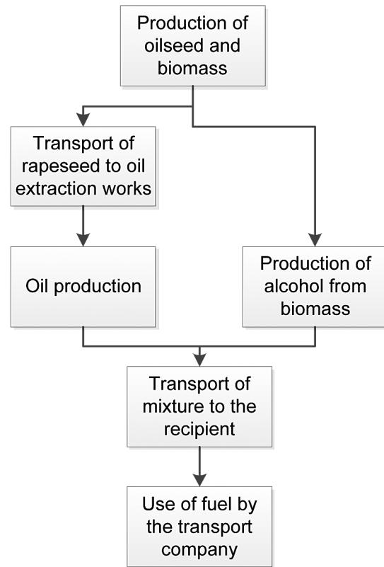
**Figure 1.** Processes of the production of life cycle of fuel mixture
