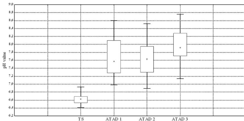
**Figure 2.** The ranges of the pH value for sludge measured during operation of a two-stage installation
