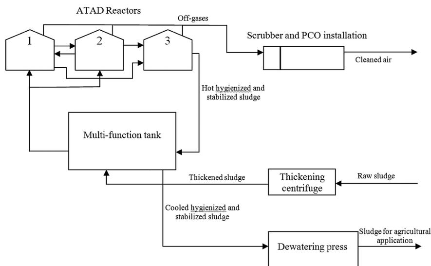
Figure 1. Simple diagram of sludge complex in Lubań wastewater treatment plant
