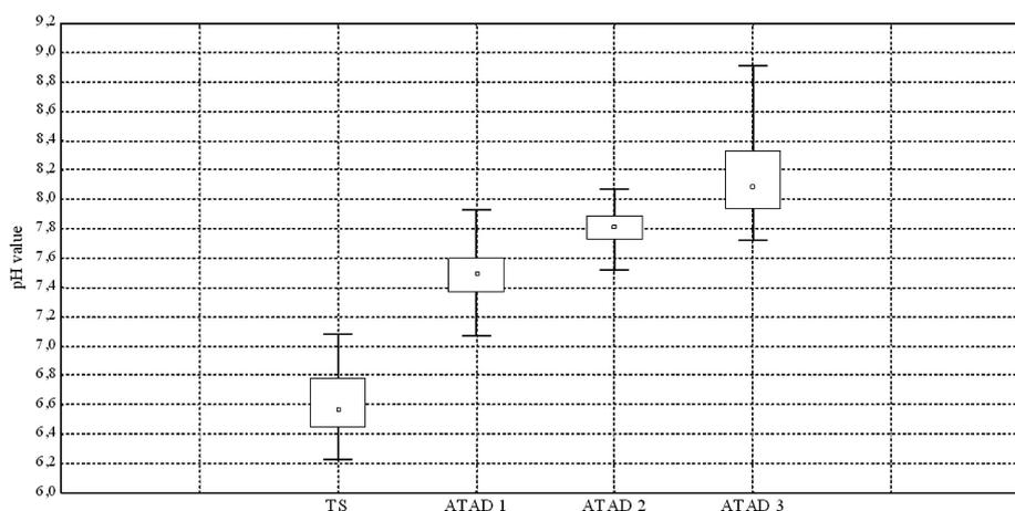
**Figure 3.** The ranges of pH value for sludge under study during operation of a three-stage installation
