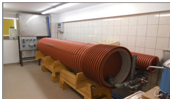
Figure 10. Fundamentals of Technology Department Laboratory – rotating biological contactor with bi-directional longitudinal flow
