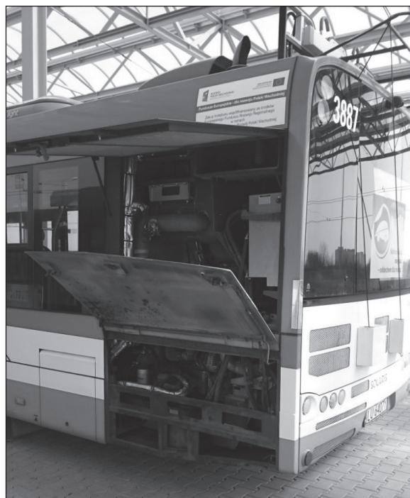
Fig. 4. The tower mounted autonomous drive system in the SOLARIS Trollino12 trolleybus.
