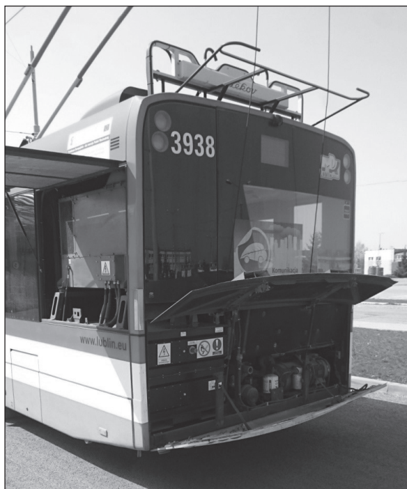
Fig. 3. The tower mounted autonomous drive system in the SOLARIS Trollino18 trolleybus.
