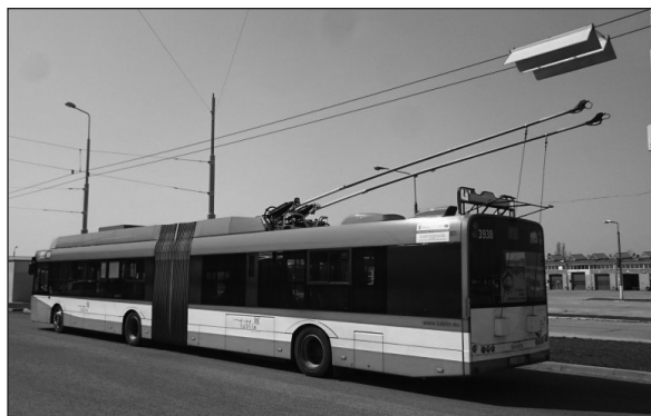
Fig. 7. Automatic connection of a SOLARIS Trollino18 trolleybus to the catenary.
