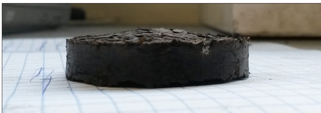
Figure 10. The swollen briquette produced at a temperature of 300 °C, at a pressure of 216 MPa
