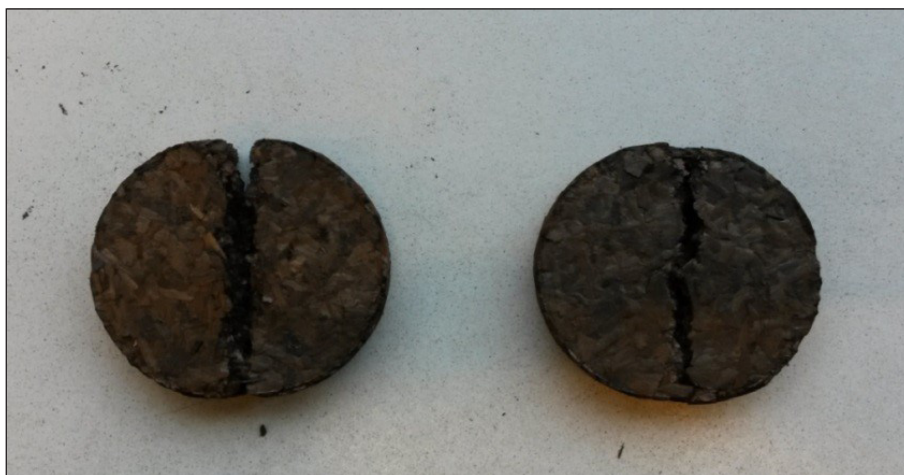
Figure 6. Briquettes after completion of strength tests
