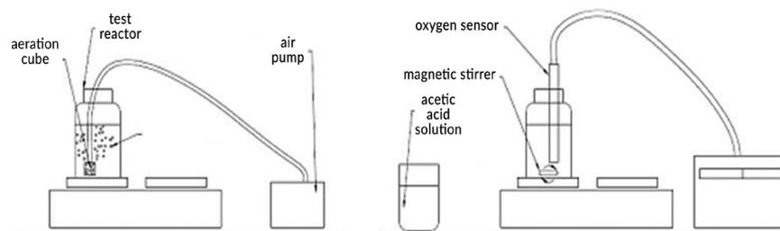
**Figure 2.** Scheme of the research stand for conducting the OUR tests.
