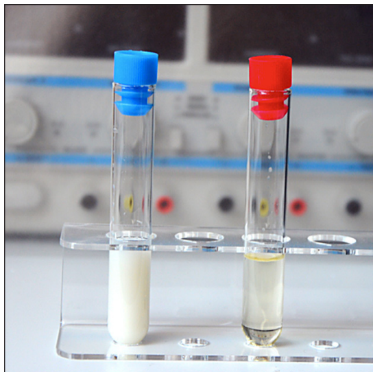
Figure 1. Coconut oil at temperature 293K (blue stopper) and at 303K (red stopper)
