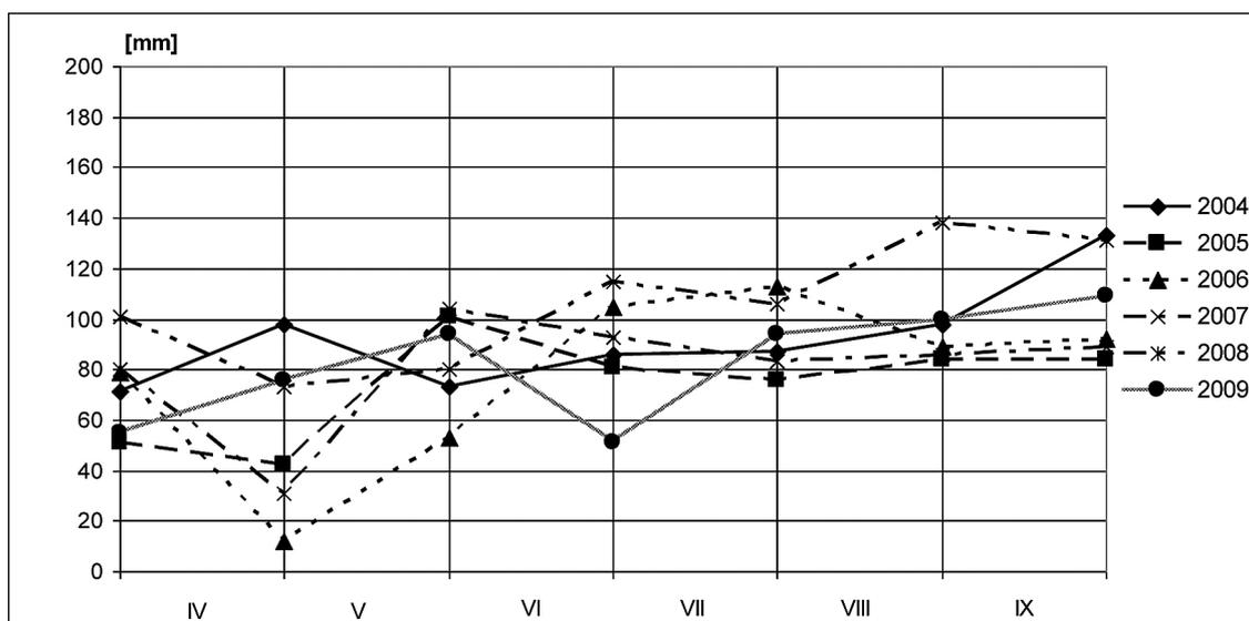
Figure 4. Differences in water reserves [mm] between soil profiles up and down the dam in 50–100 cm stratum
