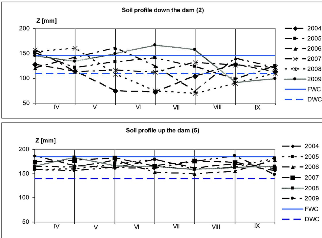
Figure 2. Water reserves in 0–50 cm soil stratum Z [mm] in soil profiles down and up the dam in vegetation periods in years 2004–2009 against the field water capacity (FWC) and drought water capacity (DWC).
