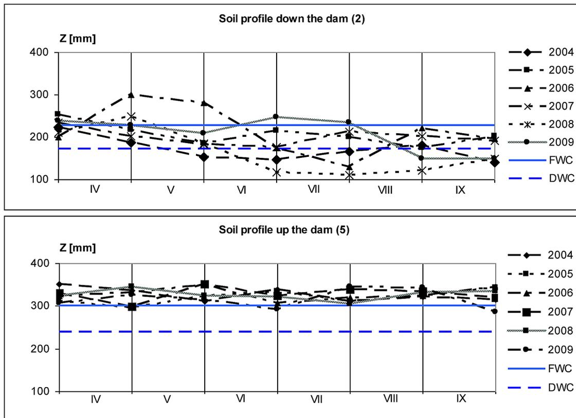
Figure 3. Water reserves in 0–100 cm soil stratum Z [mm] in soil profiles down and up the dam in vegetation period in years 2004–2009 against the field water capacity (FWC) and drought water capacity (DWC)
