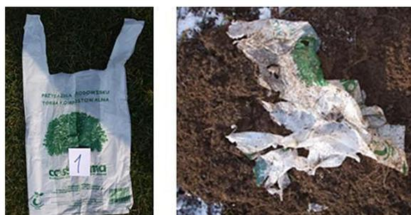
**Figure 10.** Sample 1 before and after the experiment – the orchard
