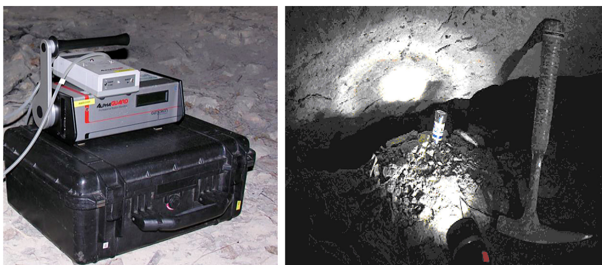
Figure 1. Measurements of radon concentrations carried in one of the caves using AlphaGUARD and passive CR-39 detector
