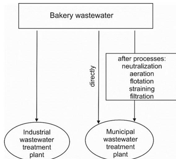
**Figure 1.** The possibilities of bakery wastewater treatment and co-treatment
