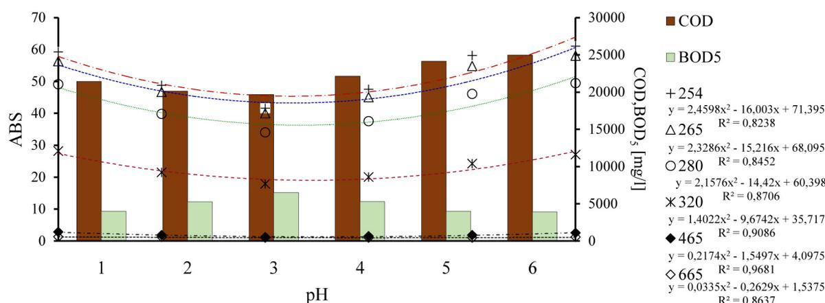
**Figure 4.** Changes in concentrations of organic compounds (COD, BOD<sub>5</sub>), including humic substances (deferent optical density) in reverse osmosis-derived retentate treated by chemical advanced oxidation with Fenton's reagent
