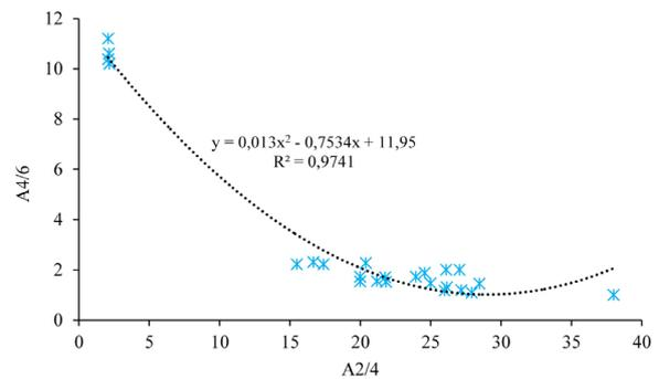
**Figure 6.** The relationships between A2/4 and A4/6 ratio in outflows after chemical oxidation of RO concentrate
