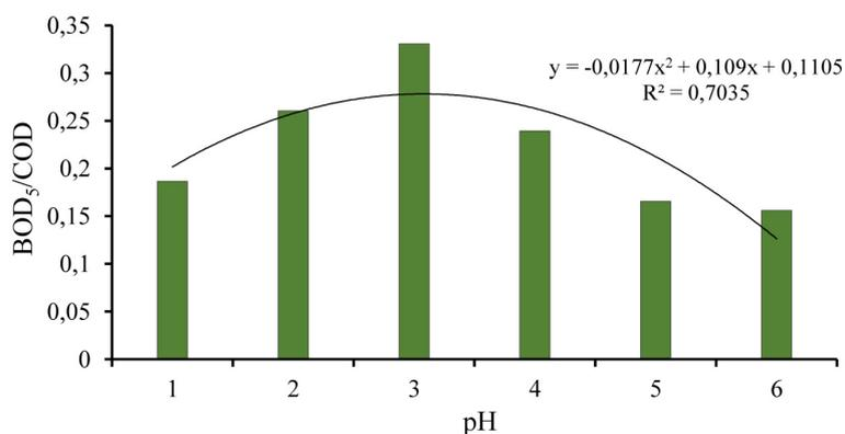
**Figure 1.** Ratio of BOD5 to COD in reverse osmosis retentate after the AOP treatment
