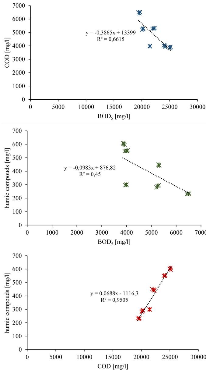
**Figure 3.** The relationships between analyzed parameters of organic carbon and the content of humic compounds in outflows after chemical oxidation of RO concentrate
