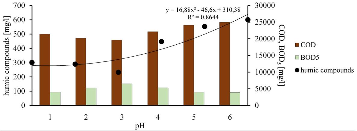
**Figure 2.** Changes in concentrations of organic compounds (COD, BOD<sub>5</sub>), including humic compounds in reverse osmosis-derived retentate treated by chemical advanced oxidation with Fenton's reagent
