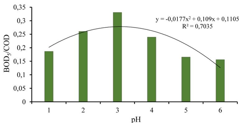
**Figure 1.** Ratio of BOD<sub>5</sub> to COD in reverse osmosis retentate after the AOP treatment
