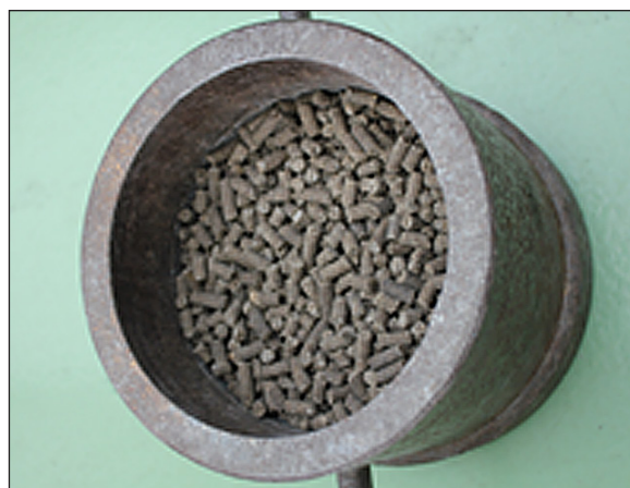
Figure 1. Sample of the examined fertilizer in the mortar before the durability test (Photo: D. Gil)
