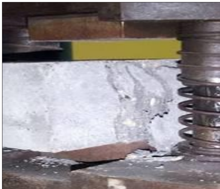
Photo 4. View of a sample subjected to compressive strength testing
