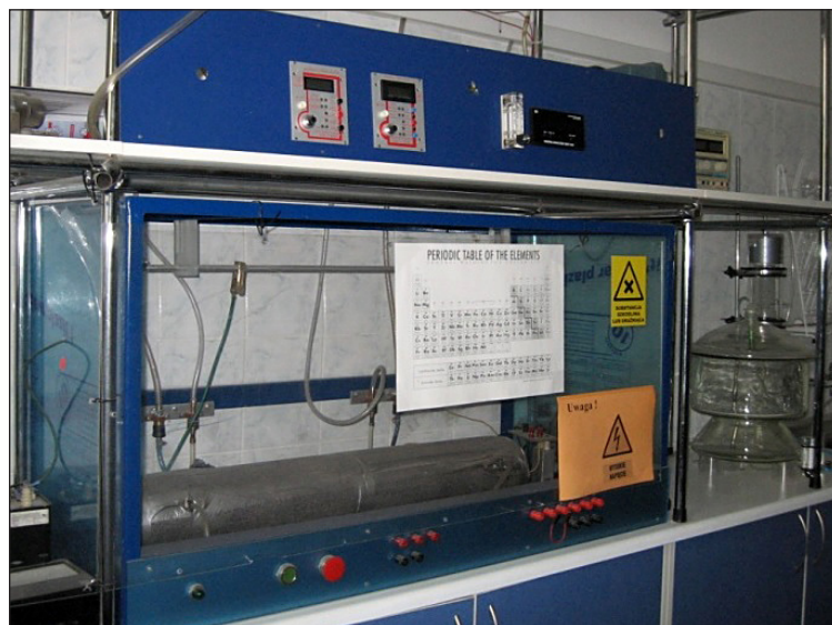
Fig. 4. Construction materials ozonation station
