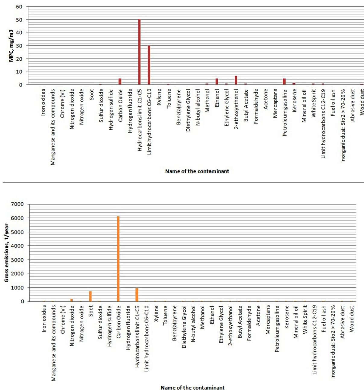
Fig. 4. Characteristics of gross emissions of pollutants from operating facilities of the gas processing plant
