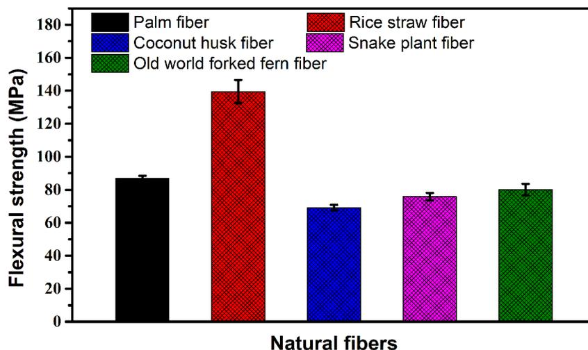
Figure 5. Histogram of the flexural strength of PP composite with different reinforced natural fibers
