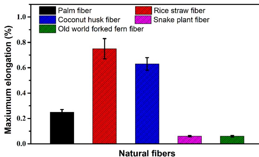
Figure 3. Maximum elongation of PP composite with different reinforced natural fibers
