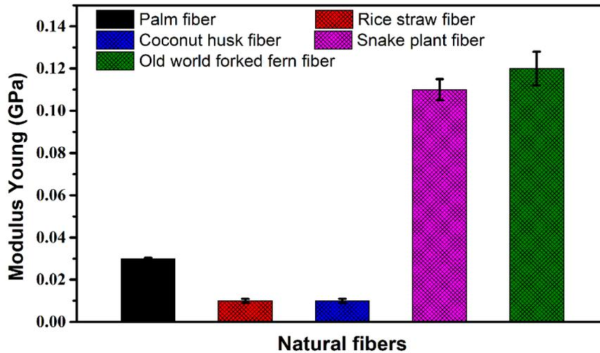
Figure 4. Modulus Young of PP composite with different reinforced natural fibers
