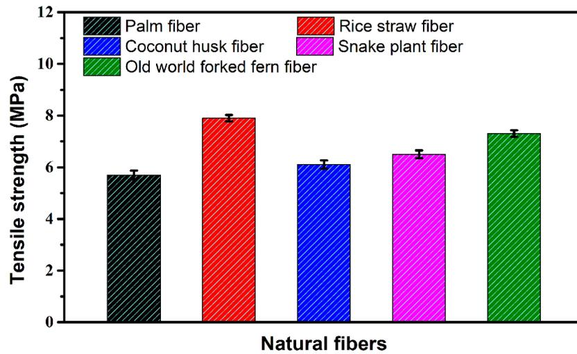
Figure 2. Histogram of tensile strength of PP composite with different reinforced natural fibers
