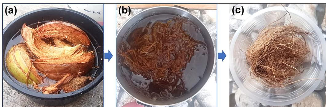
**Figure 1.** Preparation of natural coconut fiber (a) coconut husk soaked in water, (b) the soft coconut husk soaked into NaOH solution, and (c) the dried coconut husk fiber
