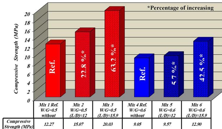
**Figure 3.** The influence of copper fibers to strengthen pure gypsum mixtures through the aspect ratio (for two different diameters) and the water/gypsum ratio
