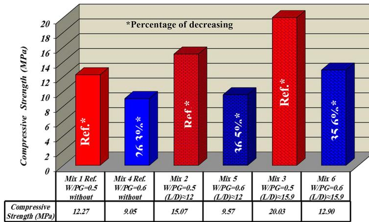
Figure 4. Effect of variable aspect ratios and W/G ratio at compressive strength of the mixture
