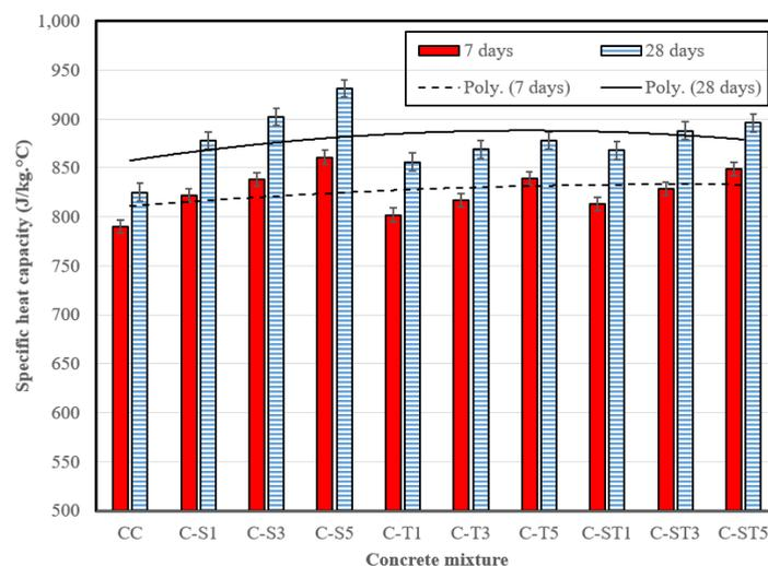
Figure 5. Mean specific heat capacity (*C* coefficient) measurements of concrete specimens
