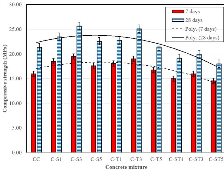
Figure 8. Mean compressive strength coefficient measurements of concrete specimens
