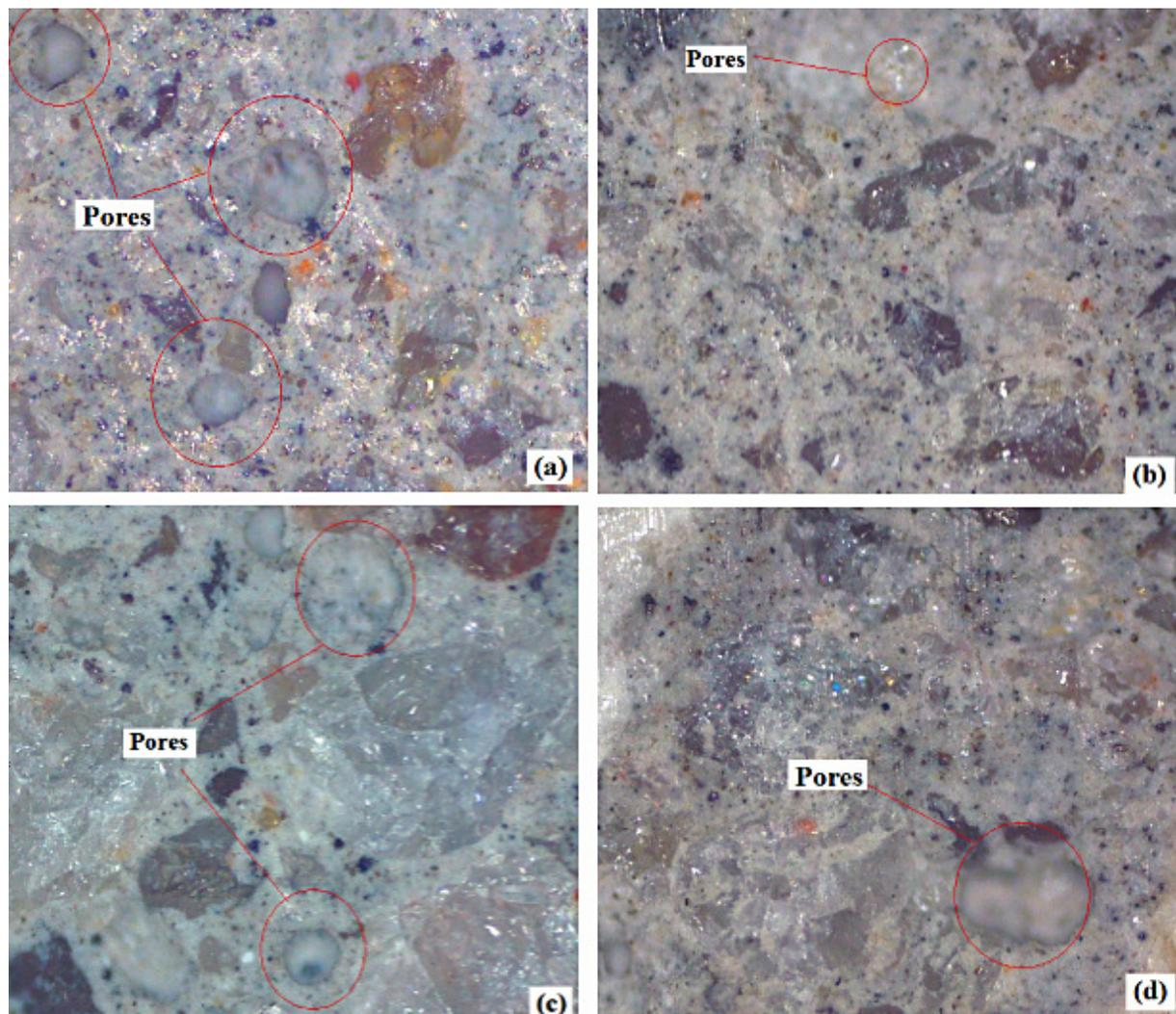
**Figure 9.** Microscopic images of concrete with (a) 0% nanoparticles, (b) 5% of nano-SiO<sub>2</sub>, (c) 5% of nano-TiO<sub>2</sub>, and (d) 2.5% of nano-SiO<sub>2</sub> and 2.5% of nano-TiO<sub>2</sub>
