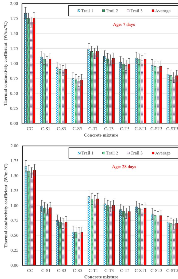
**Figure 3.** Repeatability of the thermal conductivity coefficient ( $k$  coefficient) measurements of concrete specimens
