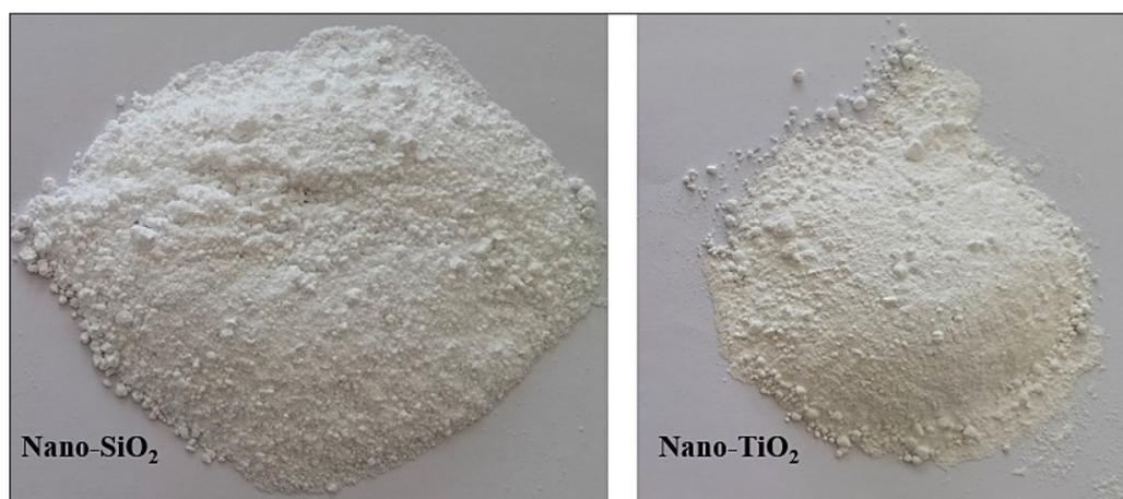
**Figure 1.** Samples of nano-SiO<sub>2</sub> and nano-TiO<sub>2</sub> materials with a particle size of 20–30 nm
