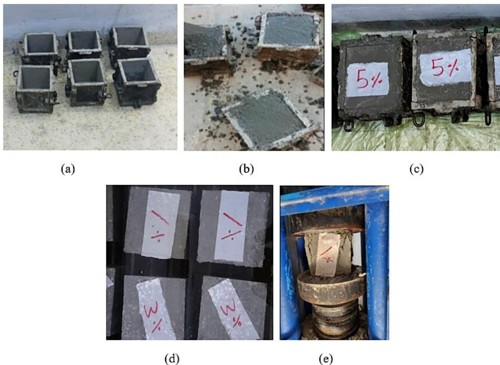
**Figure 2.** Photos of experiments: (a) models before casting, (b) casting of samples, (c) models after casting, (d) samples in the duration tank, and (e) shape of the failed sample
