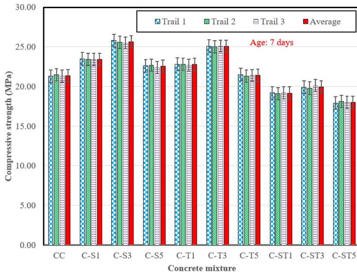
Figure 7. Repeatability of the compressive strength coefficient measurements of concrete specimens
