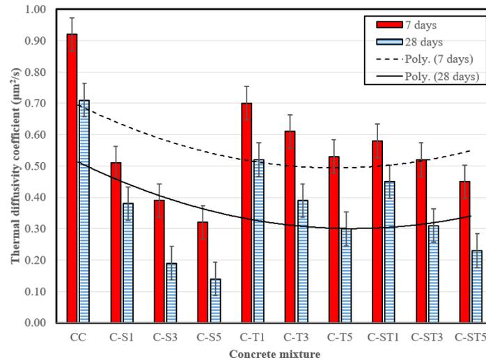
**Figure 6.** Mean thermal diffusivity coefficient ( $\alpha$  coefficient) measurements of concrete specimens
