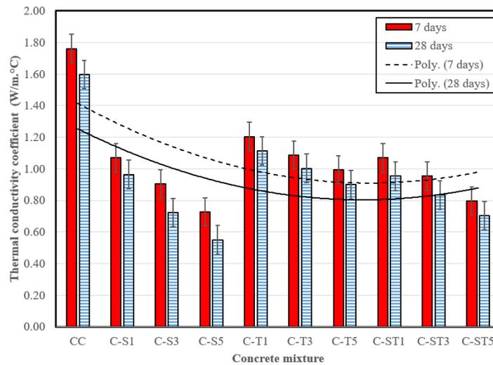
Figure 4. Mean thermal conductivity coefficient (*k* coefficient) measurements of concrete specimens
