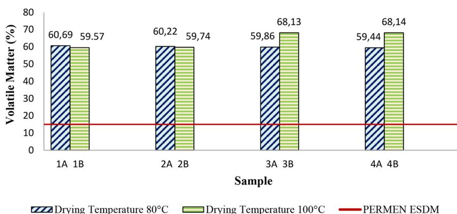
Figure 5. Concentration of volatile matter in Sungkai sawdust biobriquettes
