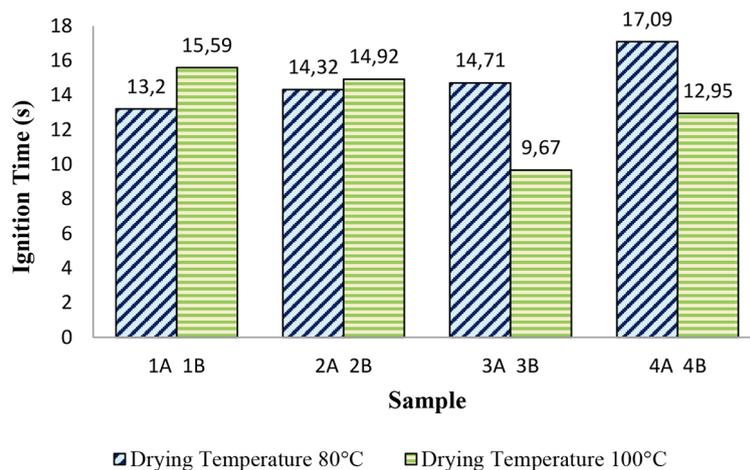
Figure 9. Ignition time of Sungkai sawdust biobriquette
