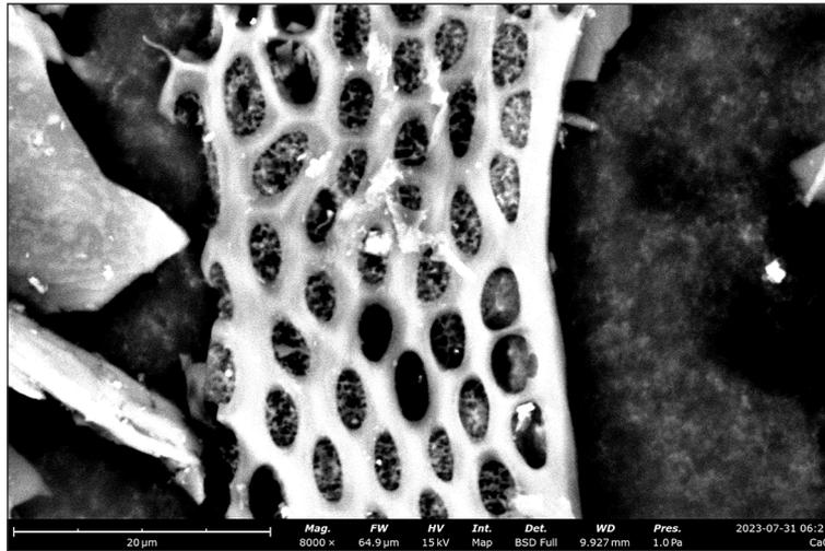
Figure 1. SEM characterization of pure Sungkai wood sawdust
