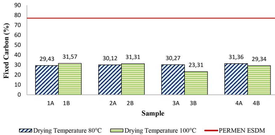
Figure 6. Carbon content of Sungkai sawdust biobriquettes
