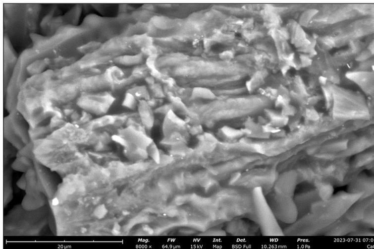
Figure 2. SEM characterization of Sungkai sawdust briquette
