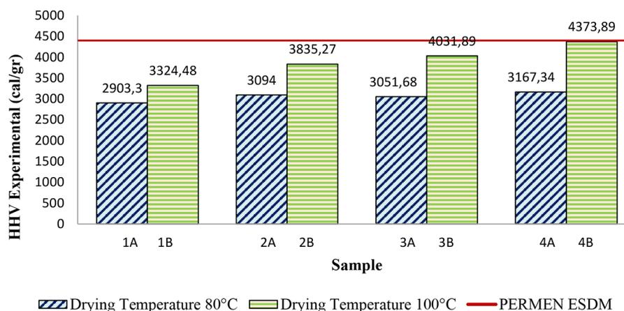
Figure 7. Experimental calorific value of Sungkai sawdust biobriquette
