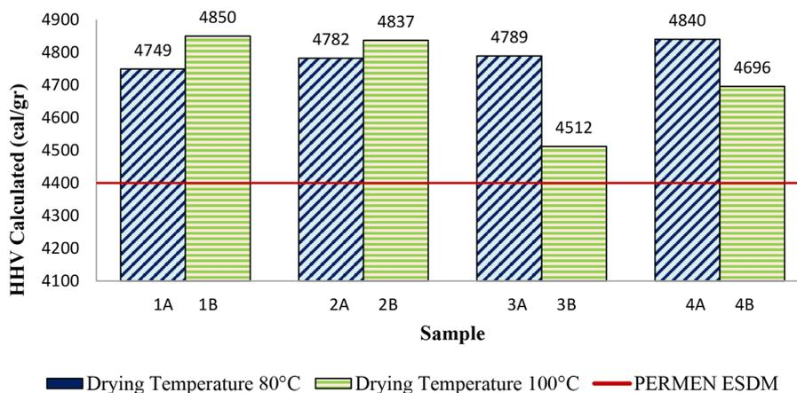
**Figure 8.** Calculated calorific value of Sungkai sawdust biobriquette
