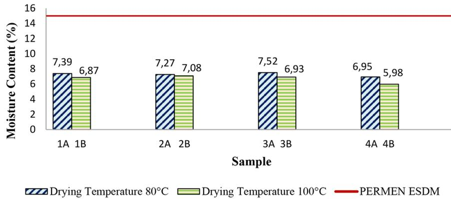
Figure 3. Moisture content of Sungkai sawdust biobriquettes
