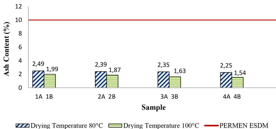
Figure 4. Ash content of wood sawdust biobriquette
