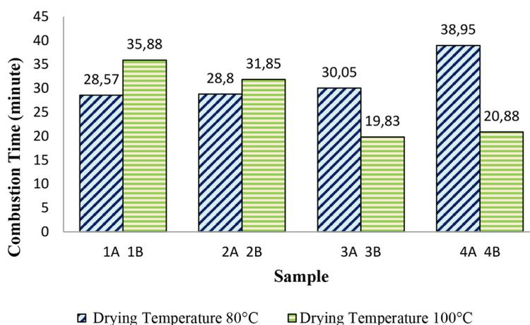
Figure 10. Combustion time of Sungkai sawdust biobriquettes
