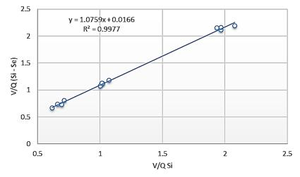
Figure 3. Stover-Kincannon modified model for COD removal in the TAMR reactor
