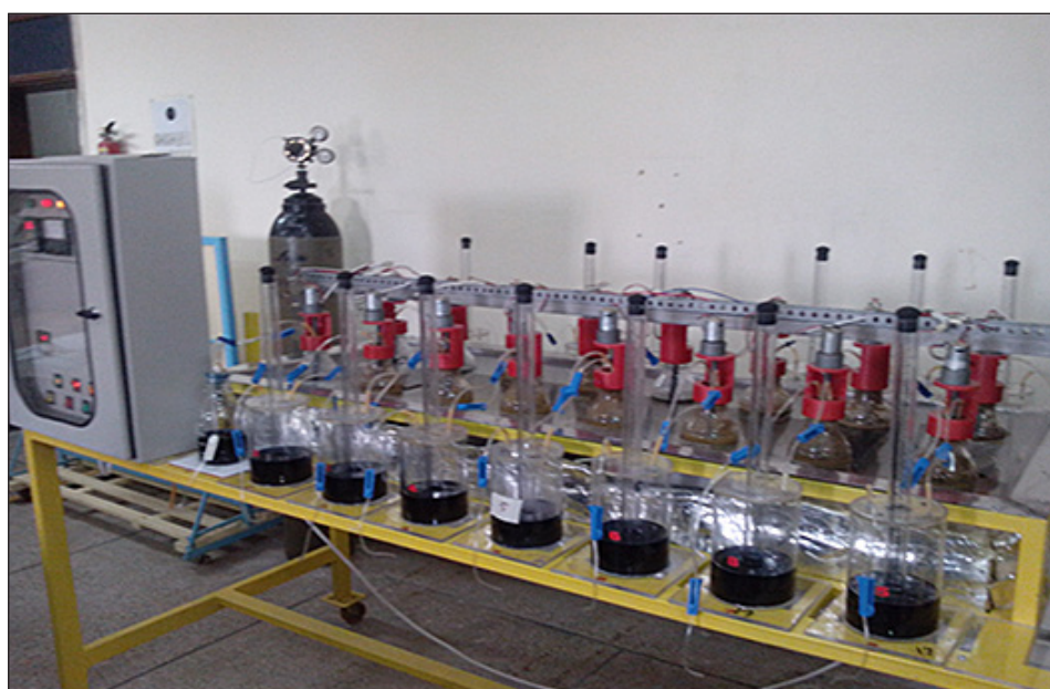
Figure 1. Semi-automatic methane potential test system
