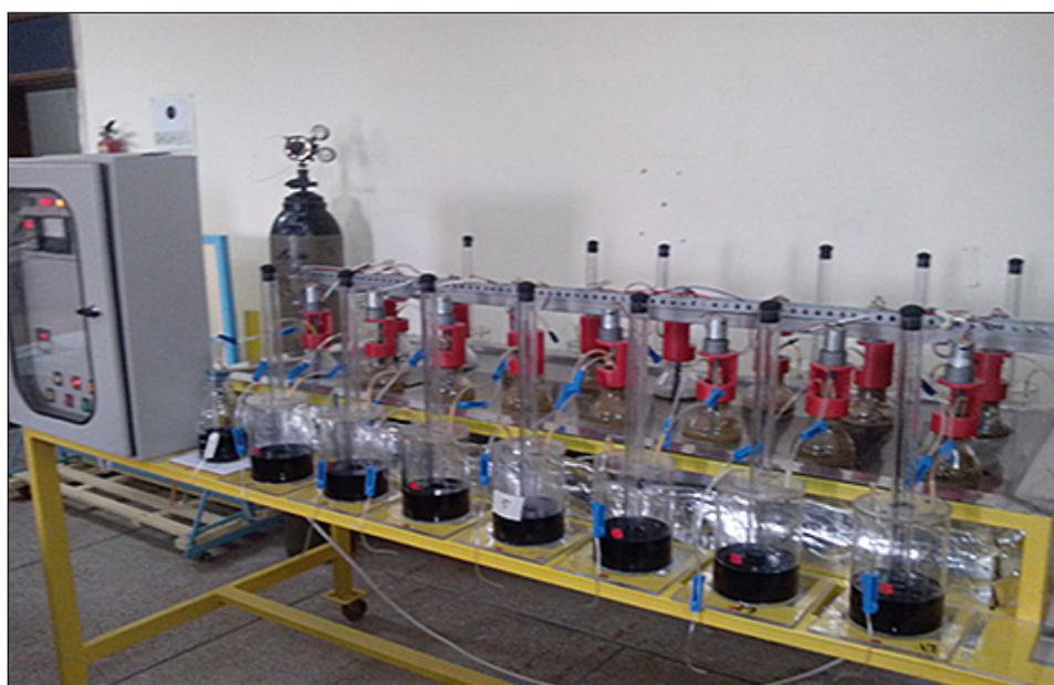
Figure 1. Semi-automatic methane potential test system
