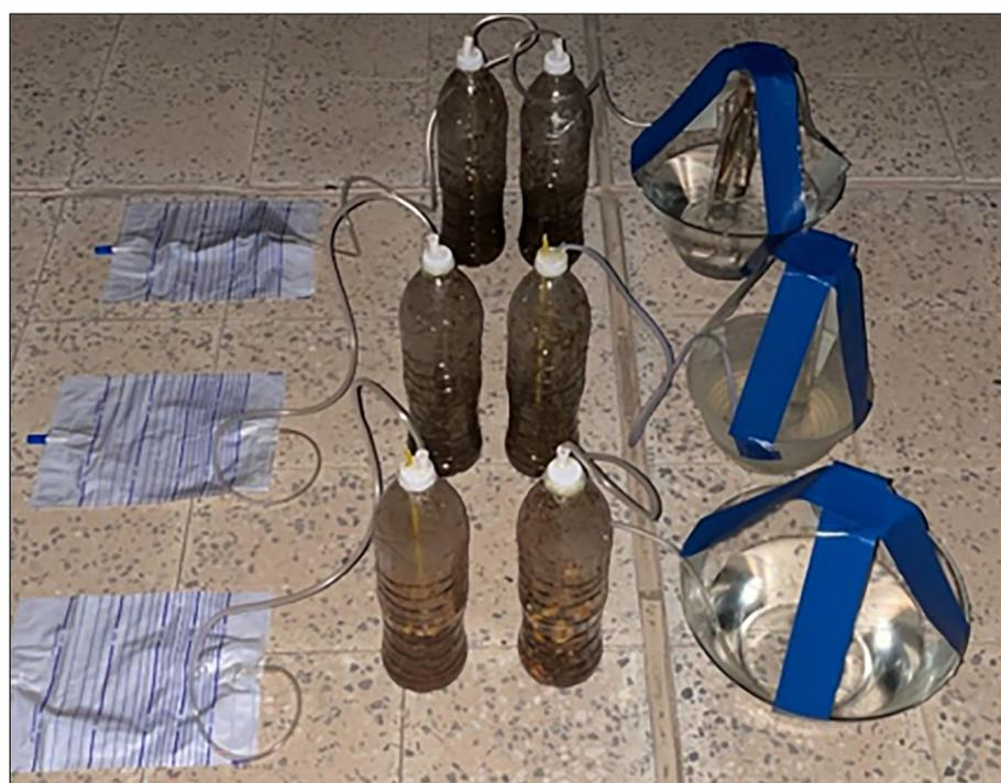
**Figure 1.** The experimental set-up of anaerobic biodigester
