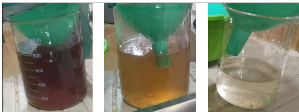
Figure 1. Filtrate colors of samples: (a) untreated; (b) pretreated KOH, (c) pretreated KOH microwave
